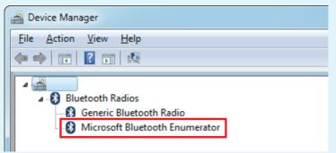
When a Windows<sup>®</sup> non-standard Bluetooth stack is used, the model name and serial number are not displayed. Make paring and virtual COM settings in the software provided with the Bluetooth stack and then register the wireless loggers. When an unauthorized virtual COM is registered, the operation of Wireless Logger Collector may become unstable.
