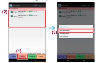
6 Collect measurement data using Wireless Logger Collector. (p. 108)
