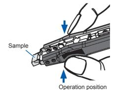
Apply an appropriate amount of force at the position shown in the figure to squeeze the pincher arms around the sample. The contact resistance value will vary with the amount of force applied. The effect of contact resistance is particularly pronounced when measuring low-impedance elements or performing short correction.
