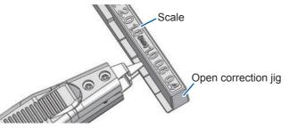
**3** Perform correction with the measuring instrument.
