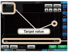
The sweep point matching the condition is indicated by a bar (|) below the X axis.
