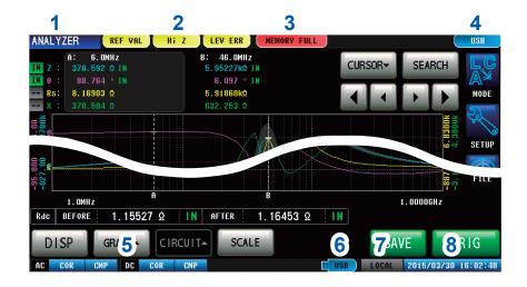
1 Displays the current measurement mode.
