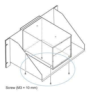
5 Use the screws removed from the legs (M3 × 10 mm) and the corresponding screw holes to fasten the instrument.
