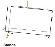
Enables the instrument to be tilted.
