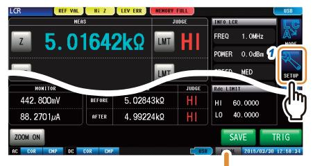
On LCR mode screen, press [SETUP] of the menu key.
