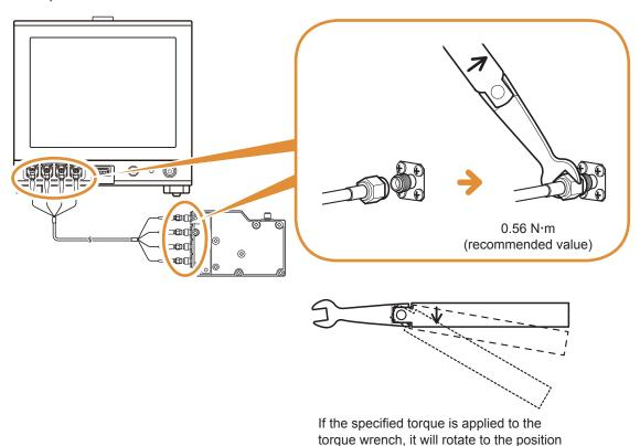
Do not rotate the cable when connecting the SMA connector of the cable to the instrument and the test head. If the cable is rotated while connecting the connector, the core wires of the connector or cable may get damaged. Rotate the nut of the connector and connect.
