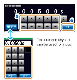
6 Set the output method to [PULSE] before setting the output time.
