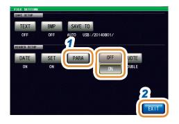
1 Select record or no record for measurement parameter in a text file.
