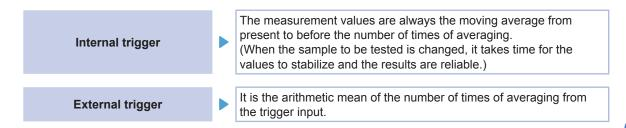
When averaging is executed 4 times, the number of measurements, measurement output points, and measurement value calculation method during output are as follows.
