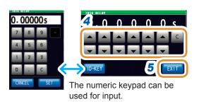
Set the delay time with ▲/▼ or with the numeric keypad.
