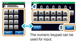
Set the wait time for switching the measurement with ▲/▼ or the numeric keypad.
