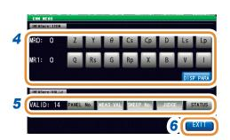
4 Select the parameters required for the measurement value. (Multiple items can be selected.)
