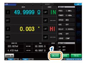
1 Press [UNLOCK] when the key-lock is enabled.
