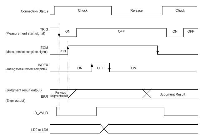
EOM: OFF From trigger to the end of measurement. INDEX: OFF Probe chuck period (Do not disengage the probe.)
