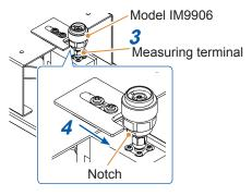
3 Place the notch of the model IM9906 Adapter parallel to the metal fittings, then install onto the measurement terminal of the test head.
