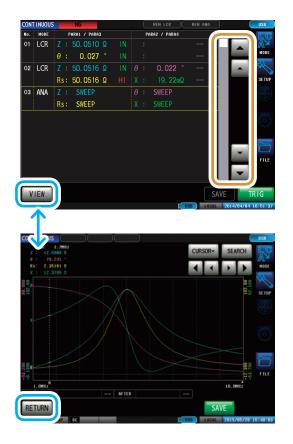
Select ANALYZER mode panel with ▲/▼ and press [VIEW].
