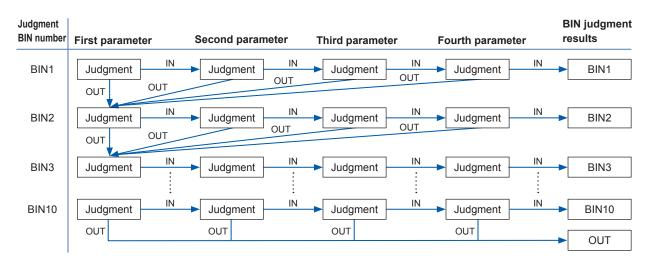
The measurement elements can be ranked by setting a series of judgment standards from severe to lenient as shown in the following diagram.
