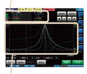
Displays the measurement results in a graph. Use this function for measuring frequency characteristics and level characteristics.
