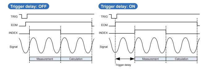
Even when the trigger delay is being used, the LED for indicating that measurement is in progress is lit.
