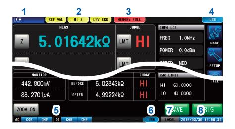
1 Displays the current measurement mode.
