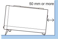
To prevent overheating, be sure to leave the specified clearances around the instrument.
