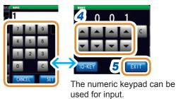
4 Set the value with ▲/▼ or the numeric keypad. (With the numeric keypad, press [SET].)
