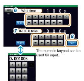
6 Use ▲/▼ or the numeric keypad to set the wait time (time to stabilize) from the time a measurement signal has been output by applying a trigger to the start of the next measurement. (With the numeric keypad, press [SET].)
