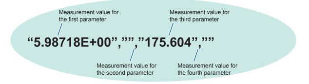
The above shows that the first parameter is "5.98718  $\Omega$ ", the third parameter is "175.604 °". Measurement values for the second and fourth parameters are not displayed as they are OFF.
