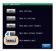
Press [MEMORY]. Measurement data is saved in the USB flash drive.
