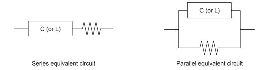
Measurement values of both modes can be displayed because the measurement value in each equivalent circuit mode is obtained by calculation. However, note that the appropriate equivalent circuit depends on the test sample.
