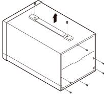
3 Remove two screws at the top of the instrument to detach the handle.
