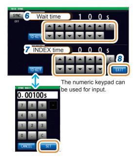
6 Use ▲/▼ to set the wait time (time to stabilize) from the time a measurement signal has been output by applying a trigger to the start of the measurement.
