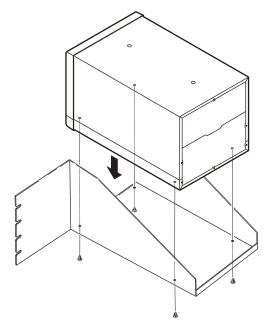
Install the spacers on both sides of the instrument, affix the rack mounting plate with the screws removed from the legs (M3 × 10 mm).
