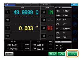
In the case of an external trigger, the key-lock is not enabled for **[TRIG]**.
