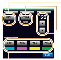
Set the waveform and the graph color for each parameter (p. 187). Settable number of colors: 25
