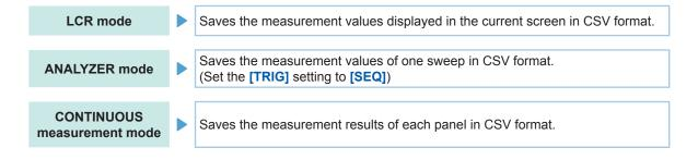
Measurement results are saved in the following order: measuring instrument information, save time and date, measurement conditions, measurement parameters, and measurement values. Text file header (save time and date, measurement conditions and measurement parameters), delimiter, and quotation mark type can be configured.
