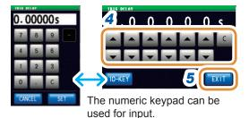
Set the delay time with ▲/▼ or the numeric keypad.
