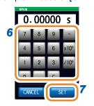
6 Set the offset delay values\* for each of the standard units of [OPEN], [SHORT], and [LOAD] with the numeric keypad.
