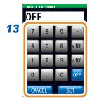
11 Use the numeric keypad to set the upper limit value of the first parameter and press [SET].
