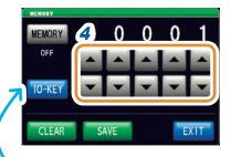
The numeric keypad can be used for input.
