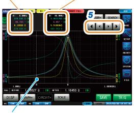
The cursor can be moved to any arbitrary position on the screen by touching the graphical display screen.
