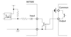
Connection with PLC output (negative common output)
