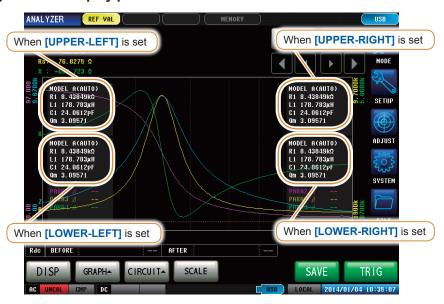
Analysis results are always shown on the upper right side for [1 X-Y] and [MULTI] display.
