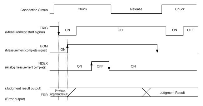
EOM:OFF From trigger to the end of measurement. INDEX:OFF Probe chuck period (Do not disengage the probe.)
