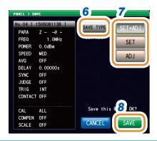
When save is executed, "PANEL SAVE" is displayed in red at the right bottom position of the screen where time is displayed.
