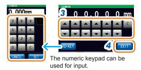
3 Set the electric length with ▲/▼ or the numeric keypad.
