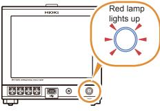
3 Put the instrument into inactive state.
