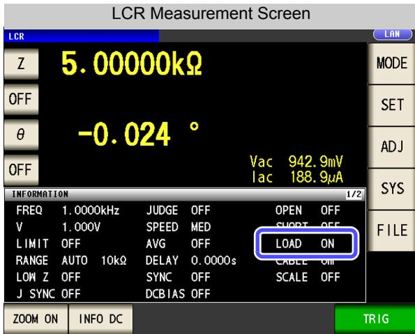
When the load compensation is valid for the set measurement conditions, ON appears on the LOAD parameter in the measurement Screen.
