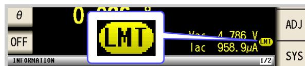
When a voltage or current in excess of the applicable limit value is not applied to the sample so that the measurement signal level setting is not reached, changes to the measurement signal level are canceled.
