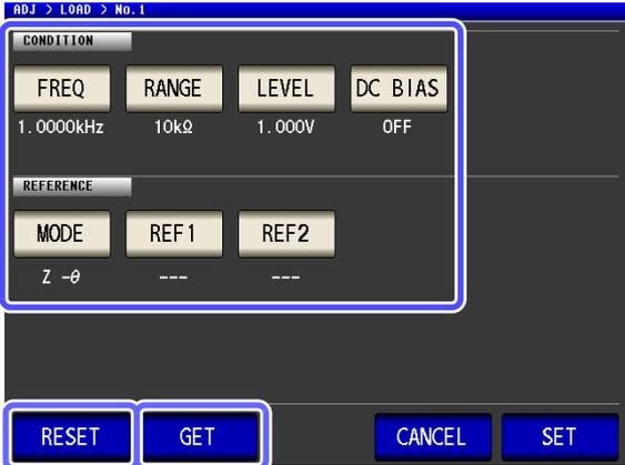
**FREQ Compensation Frequency** → Define the measurement frequency used to measure and compensate the reference sample. (p. 330)
