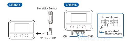
3 Set the measurement condition Measurement settings can be changed from supported instrument or Windows® PC/Android application. The settings can't be changed only by this instrument. 3 Using the LR8410 as a Unit
