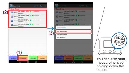
6 Collect measurement data using Wireless Logger Collector.
