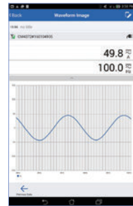
Wave Graph Simple oscilloscope No waveforms are displayed during PEAK output or with Hz function set.
