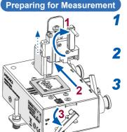
Turn the pusher up/down operation knob in the "up" direction to raise the tip pin.
