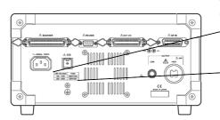
Supply voltage indicated on the rear panel (Specified at time of order)
