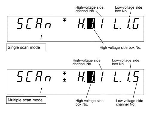
**9.** When the **ENTER** key is pressed, the **W/I** lamp lights up. Using the W key or I key, select a withstand-voltage test or insulation-resistance test to be conducted. To terminate the program test in this step, select OFF using the ON/OFF key. To continue the test, select ON. (If the step number is 50, ON cannot be selected.)
