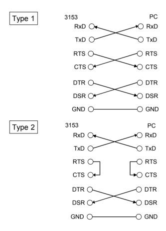
Connector on cable side: D-Sub 9 Pin female
