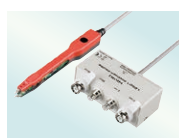
PINCHER PROBE L2001 Cable length 73 cm (2.40 ft), DC to 8 MHz, impedance characteristics of 50 Ω, 4-terminal pair configuration, tip electrode spacing: 0.3 (0.01 in) to 6 mm (0.24 in)
