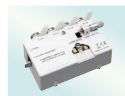
SMD TEST FIXTURE IM9110 Direct connection two-terminal measurement type for measuring SMDs, DC to 1 MHz, measurable sample sizes: 008004 (inch)
