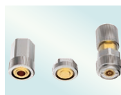
CALIBRATION KIT IM9905 Open/Short/Load set
