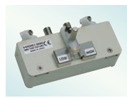
SMD TEST FIXTURE 9699 Direct connection type, For measuring SMDs with electrodes on the bottom; DC to 120 MHz, test sample dimensions: 1.0 mm (0.04 in) to 4.0 mm (0.16 in) wide, max. 1.5 mm (0.06 in) high
