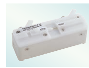
SMD TEST FIXTURE 9677 Direct connection type, For measuring SMDs with electrodes on the side; DC to 120 MHz, test sample dimensions: 3.5 mm ±0.5 mm (0.14 in ±0.02 in)
