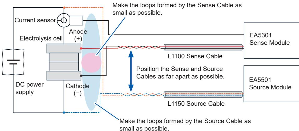
\*Twist the cables together right up to the measurement target.
