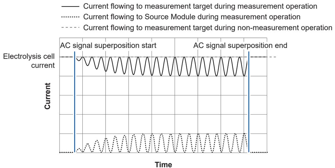
Diagram of current applied to measurement target during measurement
