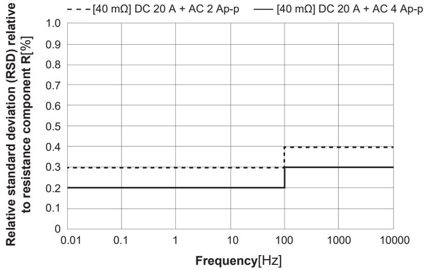
Relative standard deviation of measured resistance value when measuring resistive load (R = 40 mΩ, 20 A DC)
