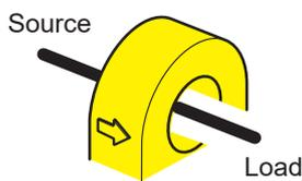
**When clamping on the positive side:**
