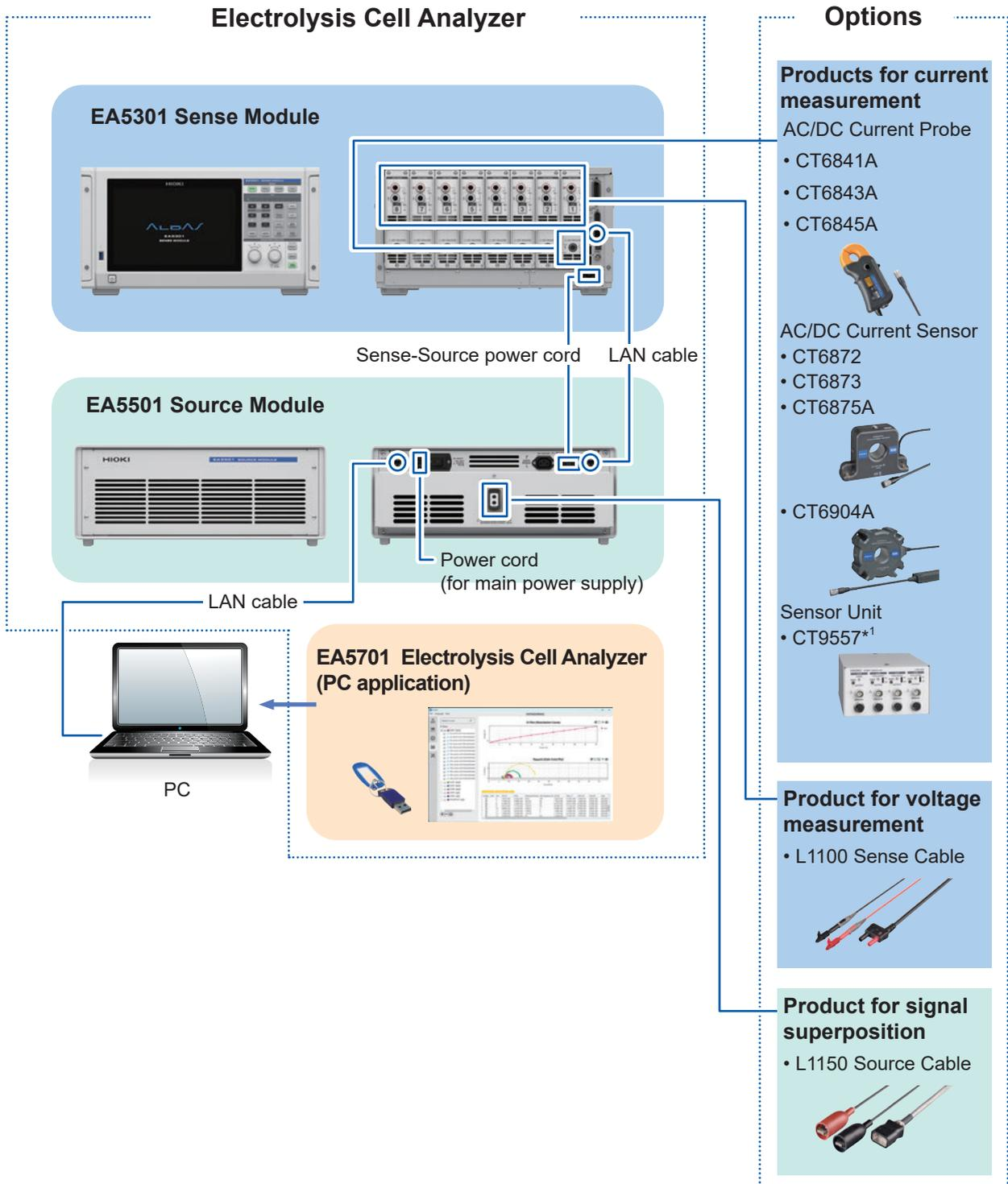
\*1. The CT9904 connection cable (optional) is required to connect to the EA5301 Sense Module.
