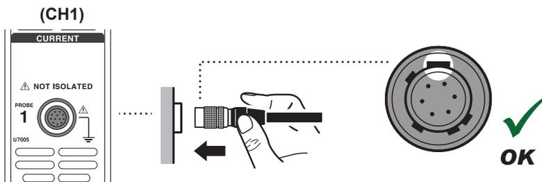
**5** Connect the connector of the L1150 Source Cable to the signal superposition terminal of the EA5501 Source Module.
