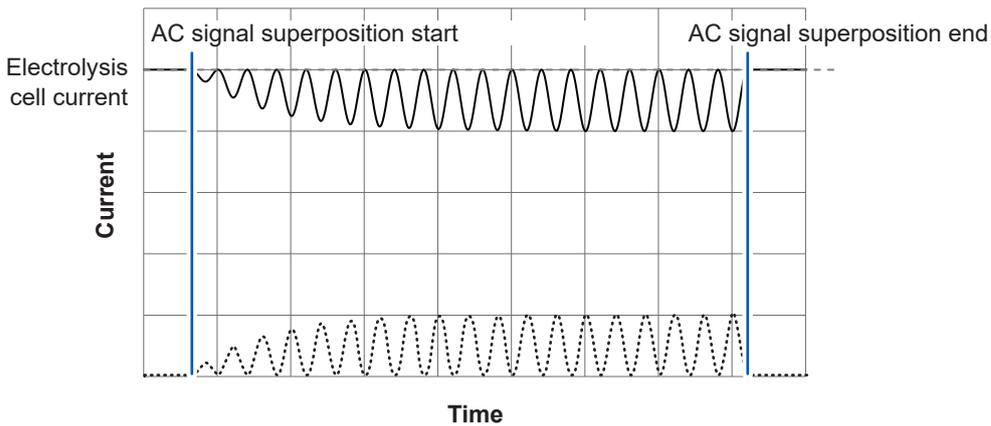
**Diagram of current applied to measurement target during measurement**
