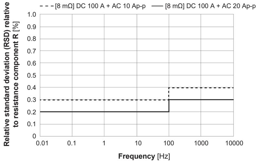
Relative standard deviation of measured resistance value when measuring resistive load (R = 8 mΩ, 100 A DC)
