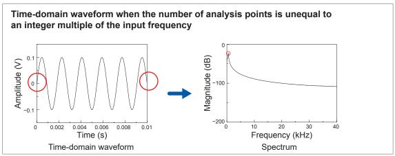
The window function has been created to suppress such leakage errors. The window function smoothly connects each cropped end of a time-domain waveform.
