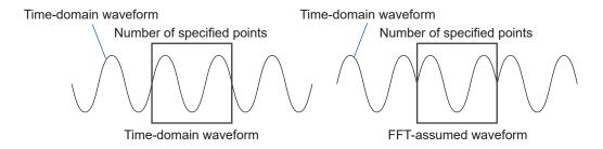
When the number of FFT calculation points is equal to an integer multiple of the input signal frequency, a single line spectrum is obtained. However, if the number is unequal to an integer multiple of the frequency (with the result that the FFT-assumed waveform has discontinuous points), spectral lines spread, resulting in failure of production of a line spectrum. This phenomenon is called the leakage error (as shown below).
