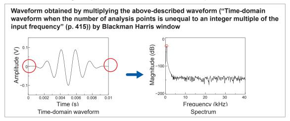
The following figure illustrate the time-domain waveform multiplied by the window function and its spectrum.
