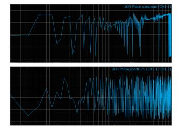
1ch FFT Horizontal axis: logarithmic Vertical axis: amplitude (linear)
