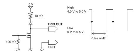
When the auto-range function is used, the instrument is triggered, outputting the TRIG.OUT signal. Be careful when performing auto-range measurement while using the TRIG.OUT signals.
