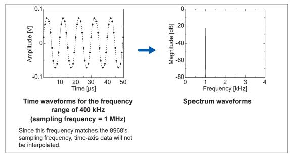
To prevent the imaging phenomenon when analyzing waveforms using the FFT function, be sure to check the unit's maximum sampling frequency prior to measurement.
