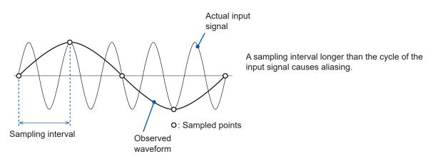
To plot a sign wave that allows you to observe the peaks without any aliasing, the instrument needs to sample the waveform at a minimum of 25 points per cycle.
