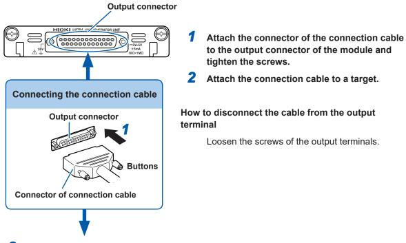
**2** Attach the connection cable to a target.
