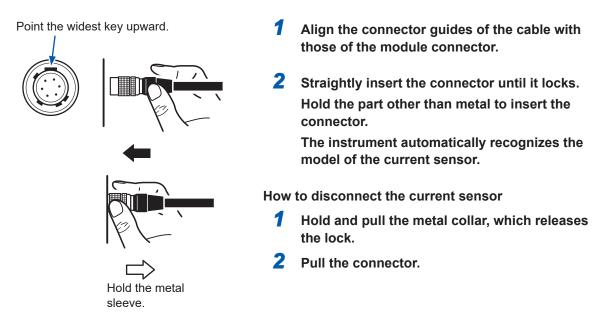
Using Model CT9900 Conversion Cable, you can connect a current sensor without the sub modelnumber "-05," which has a plastic connector (PL23), with Model U8977 3CH Current Unit.
