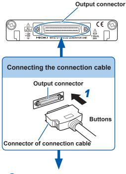
**1** Attach the connector of the connection cable to an output connector of the module.
