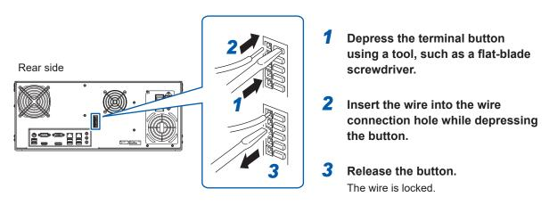
The external control terminal shares the ground with the chassis.
