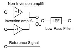
Given "v1," a reference signal voltage for the AC current generated in the instrument, and "v2," the signal voltage for use in synchronous detection, these parameters may be expressed by the equation given below.  $\theta$  of v2 shows the phase difference against v1 and is generated by the reactance.
