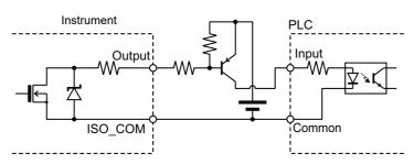
**PLC Input (Sink Input) Connections**
