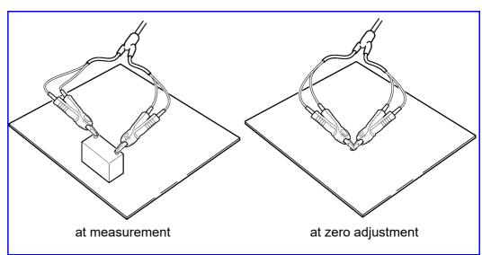
These variations are particularly pronounced in the 3 m $\Omega$  and 30 m $\Omega$  ranges, so be sure to position the leads in same state as will be used to perform actual measurement when using those configurations.
