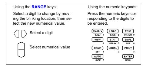
To enter the current measurement as the setting value: AUTO key (Press on a screen other than the upper/lower threshold setting display.)
