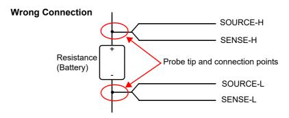
When connecting to a test object, connect SOURCE-H and SOURCE-L toward the outside, and SENSE-H and SENSE-L toward the inside.
