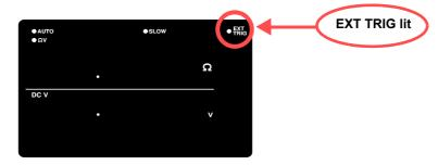
**EXT.TRIG** lit...... External triggering is selected. **EXT.TRIG** not lit....... Internal triggering is selected.
