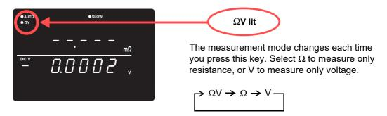
Set the measurement range. (Here, 30 m $\Omega$  range is selected.) See "3.4 Setting Measurement Range" (p.31).
