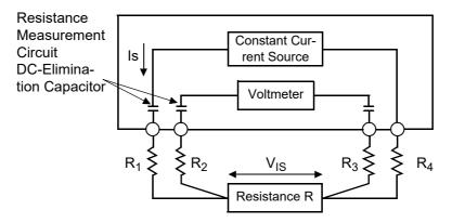
Values R1 to R4 are the resistances of the test leads plus contact resistances.
