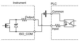
**PLC Input (Source Input) Connections**
