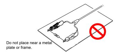
Observe the precautions illustrated in the following diagram concerning the shape and placement of measurement leads. Eddy currents and outside induced noise caused by nearby metallic objects can introduce an error component or variation into measured values, degrading repeatability. (The impact of these phenomena can be reduced as described below.)
