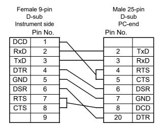
Note that the combination of a dual male 25-pin D-sub cable and a 9- to 25-pin adapter cannot be used.
