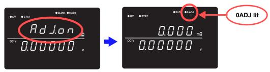
After measurement, the measured value of the compensation applied by the zero-adjust function is displayed.
