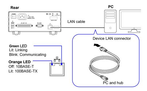
If the green LED on the LAN connector is not lit even after the device has been connected to the LAN, the device or connection device may be malfunctioning or the LAN cable may have a broken wire.
