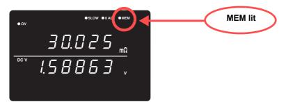
If an external trigger source is selected, one measurement is stored after each trigger event. In the internal triggering case, the first measurement value after triggering is stored. Apply a trigger as many times as is necessary.
