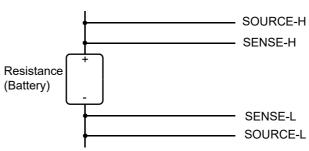
Do not allow the test leads near metal surfaces. In particular, the lead portions that are not twisted together must be kept away from conductors to avoid unstable measurements resulting from the effects of induced current.
