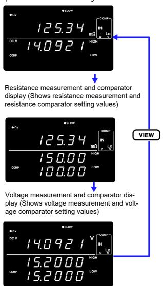
Measurement display switching is available only with the comparator enabled, and in the  $\Omega V$  mode.
