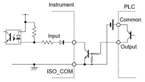
PLC Output (Source Output) Connections
