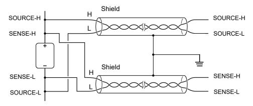
The four-terminal design requires that all four terminals be used for measurement. Attempting to measure with two terminals (the two lines in the middle) may result in unstable or inconsistent measurements due to the effects of test lead contact resistance.
