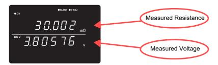
In the  $\Omega$  mode, resistance measurements appear on the upper display.
