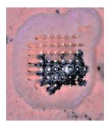
Electrode material may adhere to the probe tips, even if the SHORT and OPEN inspections yield normal results (see photograph at left). Since such deposits may cause contact defects or insulation defects or negatively affect probe movement, they must be removed immediately. Please clean the probes, referring to "Air (compressed air) cleaning" (p. 137).
