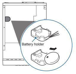
**5** Insert the tweezers into the space between the battery and the battery holder and remove the battery while lifting up on it, as shown in the figure.
