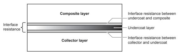
Figure: Diagram showing a cross-section of an electrode using a collector with an undercoat layer
