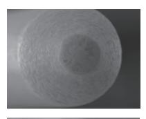
This scanning electron microscope (SEM) micrograph depicts the tip of an unused probe.
