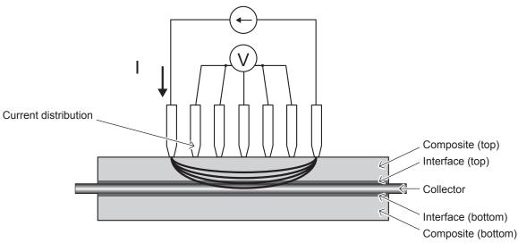
Figure: Cross-sectional diagram of measurement of double-coated electrodes
