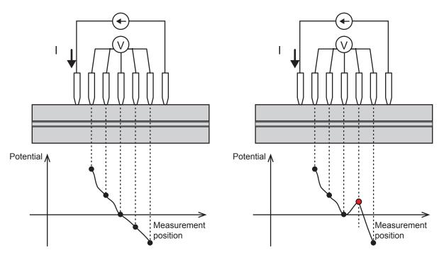
Figure: Illustration of consistency (left: PASS consistency; right: FAIL consistency)
