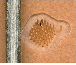
46 probes (The left object is a mechanical pencil lead [0.5 mm].)
