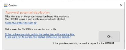
A description of how to resolve the FAIL result is shown in the window. Please refer to this information when performing probe maintenance.
