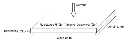
Figure: Definition of surface resistivity
