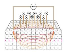
Illustration of finite volume model and equivalent resistance matrix
