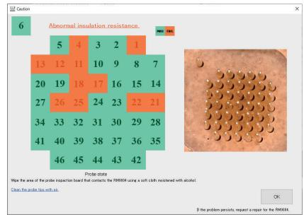
The figure on the left displays the status of each probe. PASS probes are shown in green, while FAIL probes are shown in orange.
