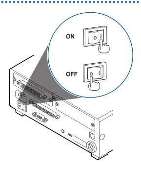
Place the RM2611 Electrode Resistance Meter's main power switch (on the rear of the instrument) in the ON (|) or OFF ( $\circ$ ) position.
