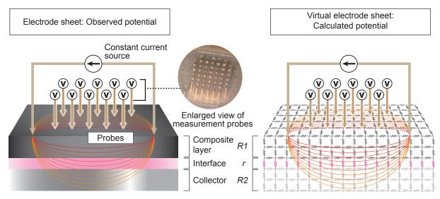
(It doesn't matter whether the electrode sheet that is measured is coated on one side or both sides. The composite layer resistivity and interface resistance on the probed surface are output.) (*R1* and *R2* thickness [µm], and *R2* volume resistivity are entered by the user.)
