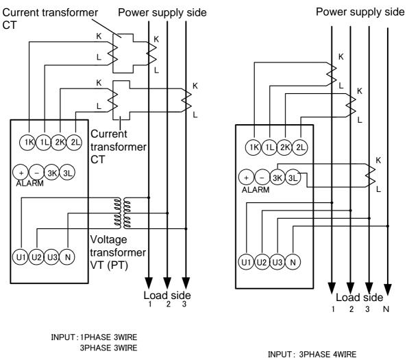
Measurement of singe-phase, 3-wire line or 3-phase, 3-wire line using CT and VT (PT) INPUT: 3PHASE 4WIRE
