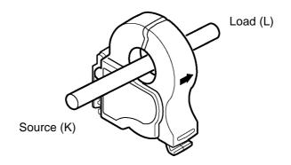
See the "Connection diagram" (P.203) and refer to the instruction manual for the clamp sensor being used.
