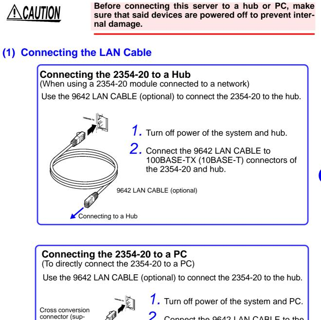
2. Connect the 9642 LAN CABLE to the cross conversion connector supplied.
