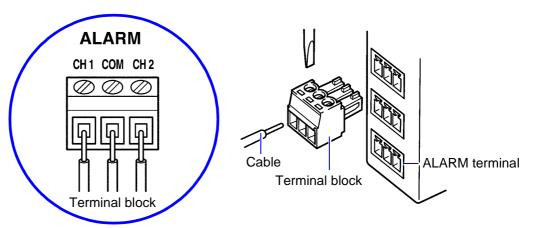
Connect the cable for CH1 output to CH1 and COM; and connect the cable for CH2 output to CH2 and COM.
