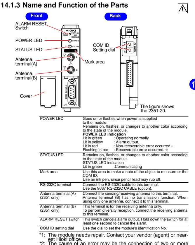
\*2: The cause of an error may be the connection of two or more communication modules. If a wireless module and LAN module are to be used, set the COM ID of the LAN module to "00."
