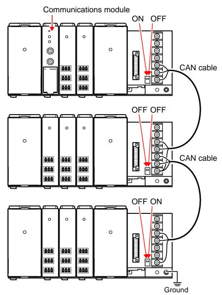
Only the CAN termination switch located on either side (a total of two) should be turned on. After all connections have been completed, check to make sure that the resistance between Hi and Lo is approx.  $60 \Omega$ .
