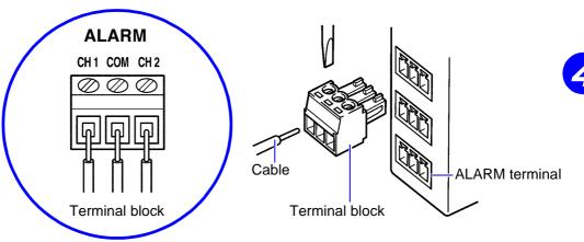
Connect the cable for CH1 output to CH1 and COM; connect the cable for CH2 output to CH2 and COM.
