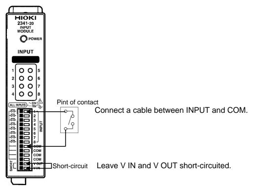
(2) Voltage Output Devices (When High Level Is +4 to 5 V)
