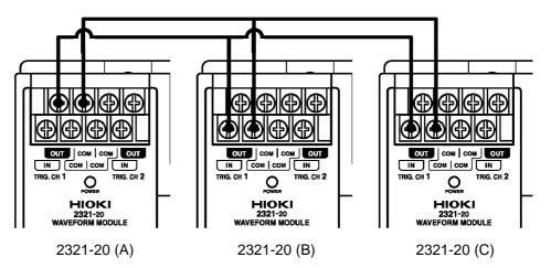
When the trigger condition for CH1 of 2321-20 (A) is met and the trigger is activated, trigger output terminal the signal for [TRIG. CH1 OUT] will change. The [TRIG. CH1 IN] of CH1 of 2321-20 (B) and 2321-20 (C) will receive the pulse signal of 2321-20 (A) and start the measurement.
