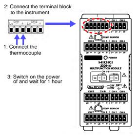
\*Alternation of the reference junction compensation between internal and external is possible
