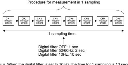
E.g. When the digital filter is set to 10 Hz, the time for 1 sampling is 10 seconds. At this time, the time lag in measurement between CH1 and CH8 is approximately 7 seconds.
