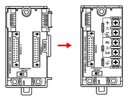
When using the 2392 MODULE BASE series, one unit of the 2392-01 must always be used.
