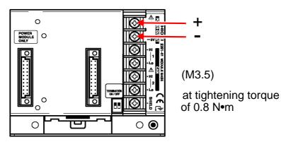
For the power supply output cable, use a cable with a conductor cross section of  $0.75 \text{ mm}^2$  (AWG18) or more and length of up to 1 meter.
