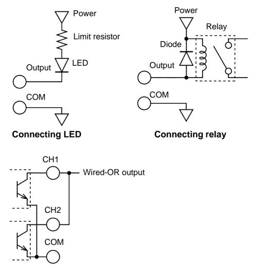
Using on Wired-OR Logic
