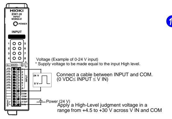
Reference: The voltage range for level judgment is as follows: H: V IN -1.0 to V IN (V) L: 0 to +1.0
