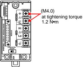
For the power supply output cable, use a cable with a conductor cross section of  $1.0 \text{ mm}^2$  or more and length of up to 1 meter (3.28 feet).
