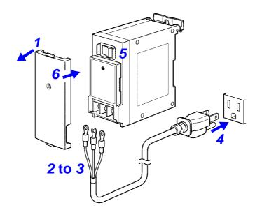
**3.** Connect the cable leads as shown below (at tightening torque of 0.8 N•m).
