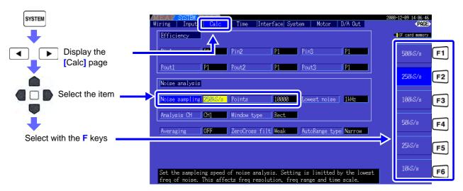
Sampling can be selected at the [Noise] setting on the [Wave + Noise] page of the Measurement screen. See How to display: "Displaying Noise" (p. 73)
