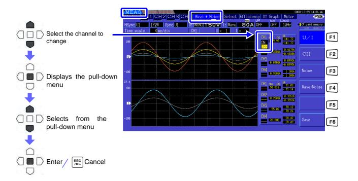
The waveform displayed on the screen or the waveform data saved in "Saving Waveform Data" (p. 118) always uses the Peak-Peak compressed waveform data sampled at 500 kS/s.
