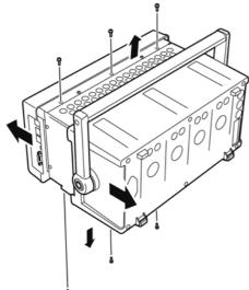
4. Remove the six Phillips head screws around the front panel, and remove the panel.
