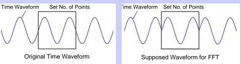
When the number of points specified for FFT calculation does not coincide with the measurement waveform period, the edges of the waveform within the window become discontinuous (called "leakage errors"), and non-existent noise is detected.
