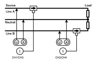
3-Phase, 3-Wire, 2-Measurement (3P3W2M)
