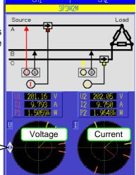
Vector line range Colors match the corresponding lines in the wiring diagram.
