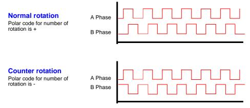
The rotation direction detected is assigned as a polar code to the measurement value of the number of rotations, and also reflected in the motor power [Pm] measurement value.
