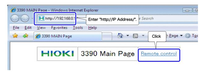
When the Main page appears as illustrated, the connection to the instrument has been established. Click the [Remote control] link to jump to the Remote Control page.
