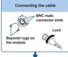
Connect the logic probe to a measurement object.
