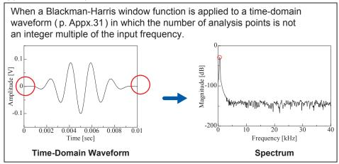
The following figure shows the time-domain waveform of the window function and its spectrum. Each spectrum shows a large peak at a low frequency, and many smaller peaks at higher frequencies. The largest peak is called the **main lobe**, and the smaller peaks are the **side lobes**.
