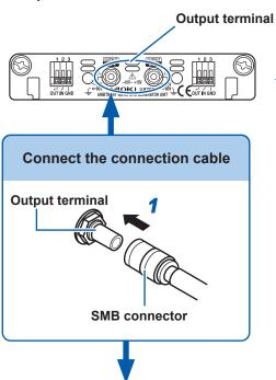
2 Connect the connection cable to an object to which the instrument applies the waveform.
