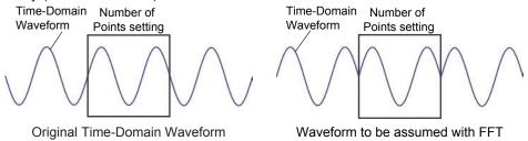
When the number of points for FFT analysis is an integer multiple of the input signal frequency, a single-line spectrum is obtained. However, if it is not an integer multiple of the frequency (When the waveform assumed with FFT includes discontinuous points), the spectrum is scattered, and a line spectrum cannot be obtained. This phenomenon is called leakage error (as shown below).
