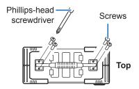
4 Remove the screws on the back side of the protectors. (8 total, top and bottom)
