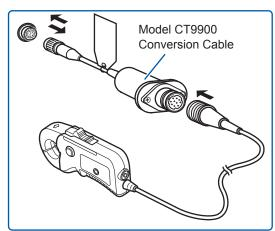
If the CT6846 or CT6865 (1000 A rating) is connected using Model CT9900 Conversion Cable, it will be recognized as a 500 A AC/DC sensor. Set the CT ratio to 2.00.
