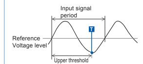
The instrument triggers when the upper threshold period elapses before the rising edge (↑ trigger slope) of the input signal crosses the reference voltage level.
