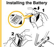
■ Press the PUSH tab as shown, and pull the battery cover back.
