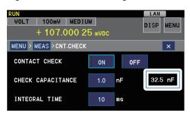
If the capacitance monitor value is the same as the contact check threshold, the instrument may either detect a contact error or display the measured value.
