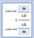
When (|measured value| ≥ lower limit value), the instrument will generate an IN judgment, including in the event of an over-range (+OvrRng/-OvrRng) event.
