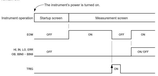
The above chart depicts instrument operation when the trigger source is set to **EXTERNAL** and EOM output is set to **HOLD**.
