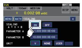
Enable the scaling function. (Default setting: OFF)
