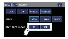
ON Automatically clears the statistical calculation results every time they are printed.
