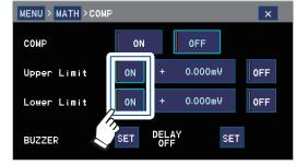
Enable upper limit and lower limit values. (Default setting: **ON**)
