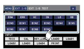
Touch the signal you wish to output. Check the connected device to verify that the signal is being output from the instrument.
