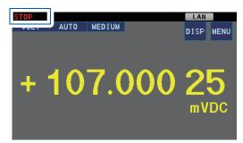
The instrument will switch to the **STOP** state.
