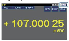
You can check the amount of available space on the USB flash drive as well as the drive's capacity on the **File** screen.
