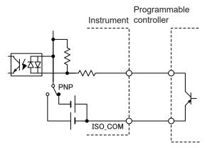
Connection to programmable controller (positive common output)
