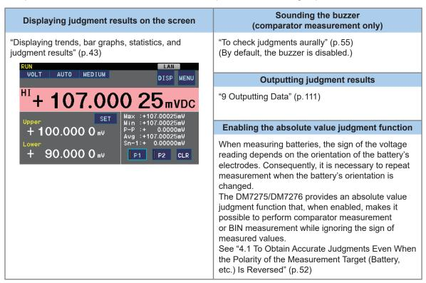
Comparator measurement and BIN measurement use the same judgment method in which measured values are compared to previously set upper limit and lower limit values. It is also possible to set only an upper limit value or a lower limit value.
