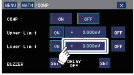
Enter a lower limit value using the same method as for the upper limit value. (Default setting: 0 V; valid setting range:
