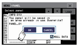
Touch **OK** to overwrite the previously saved data with the current measurement conditions.
