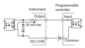
Connection to programmable controller (negative common input)
