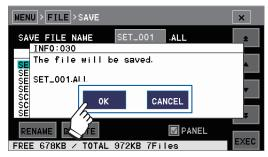
Touch **OK** to output the selected measurement conditions to the USB flash drive.
