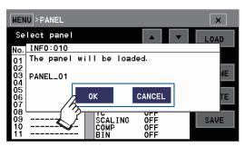
Touch **OK** to replace the current settings with the settings in the loaded panel data.
