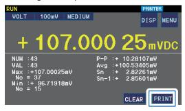
If there is no valid data, only the number of data points will be printed. If there is one valid data point, the sample standard deviation and process capability index will not be printed.
