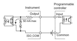
Connection to programmable controller (positive common input)
