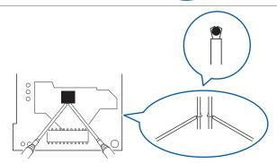
**3** Grip the measurement target with the clip.
