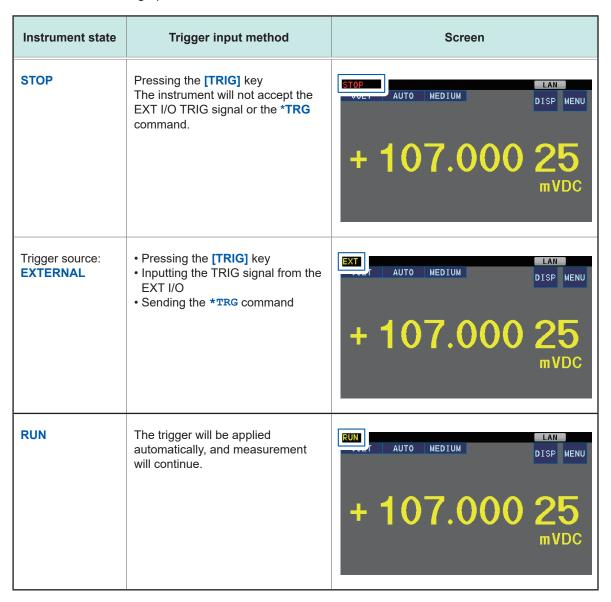
Inputting the trigger while the instrument is not in the **RUN** state will cause measurement to be performed the set number of times (the default setting is 1), after which the instrument will enter the standby state and wait for the next trigger.
