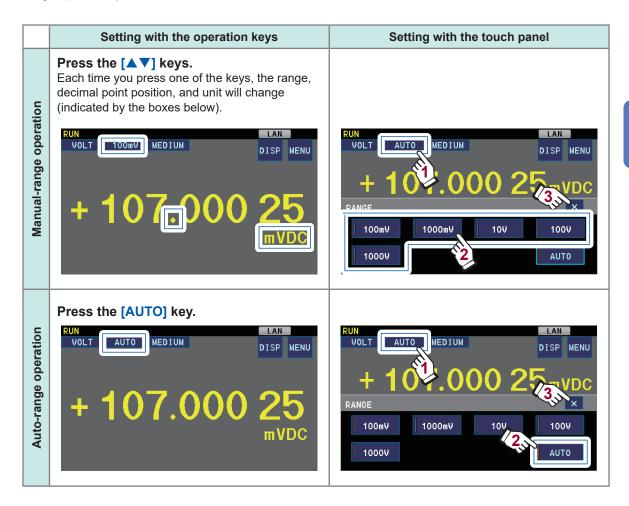
Auto-range operation may not stabilize for some measurement targets. In this case, set the range manually.
