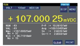
Example screen: When the BIN function and comparator function are set to **OFF** (The screen display varies with the BIN function and comparator function settings. (p.44))
