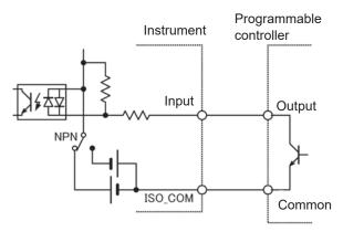
Connection to programmable controller (negative common output)
