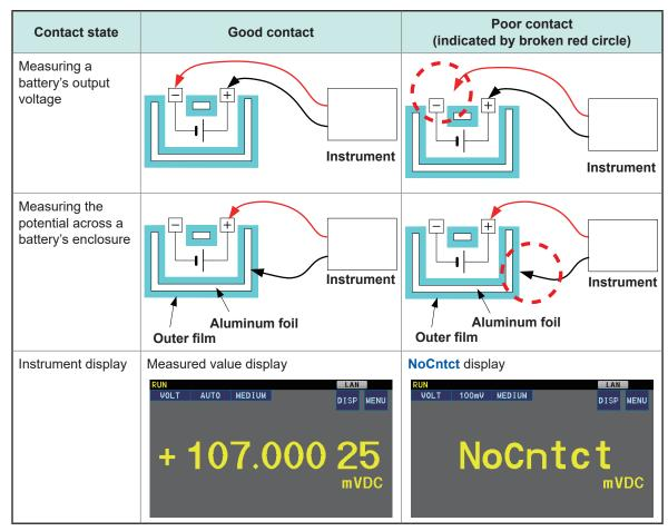
The contact check function can be used with the 10 V range and lower ranges.
