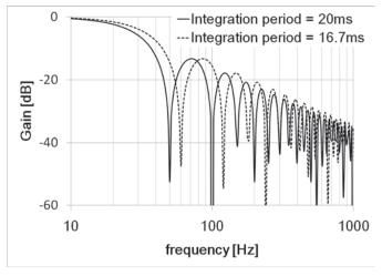
Figure 6. Noise Rejection Characteristics Using Integration
