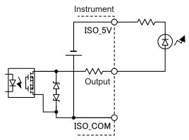
Connection to LED (using ISO\_5V, PNP setting)
