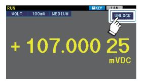
While the key lock function is enabled, the **KEY** icon will be displayed at the top of the screen.
