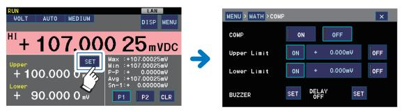
The screen display varies with the combination of comparator measurement and BIN measurement.
