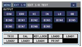
Input a signal from the connected device. The corresponding indicator will turn green to indicate the signal being input to the instrument.
