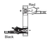
Connect, taking care to align the measurement cable colors with the measurement target's polarity. Clip at the middle of the clip.
