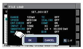
Touch **OK** to replace the instrument' settings with the loaded measurement settings.
