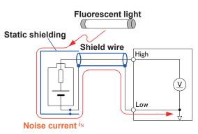
Figure 2. Noise Countermeasures Using Shielding
