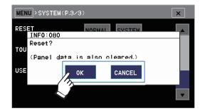
Touch **OK** to perform the reset. (Example screen: When **SYSTEM** is selected)
