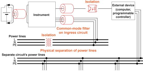
Figure 2. Conductive Noise Countermeasures
