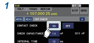
Enable the contact check function.
