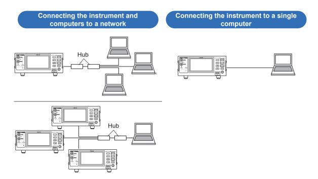
In addition, you can control the instrument using communications commands by creating a program and having it connect to the communications command port using TCP. (See the Communication Command Instruction Manual on the included application disc.)
