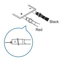
Connect, taking care to align the measurement cable colors with the measurement target's polarity.
