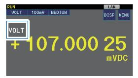
Labels cannot be displayed when the auto-hold function (p.70) is enabled.
