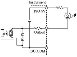
Connection to LED (using ISO\_5V, NPN setting)
