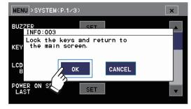
The key lock function will be enabled, and the display will return to the Measurement screen.
