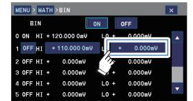
Enter a lower limit value using the same method as for the upper limit value.
