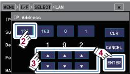
Set the IP address, subnet mask, gateway, and communications command port.
