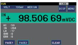
The count for each judgment result, the number of measured values outside the measurement range, and the number of errors are shown.
