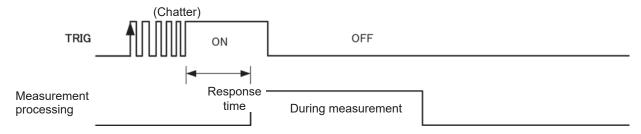
Hold the input signal until the response time has passed.
