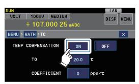
Enable the temperature compensation function.
