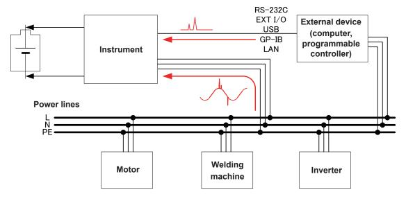
Figure 1. Ingress of Conductive Noise
