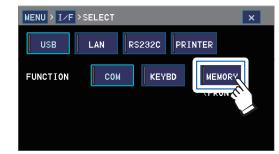
When USB COM or USB KEYBD is selected, data cannot be saved on a USB flash drive.
