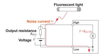
Figure 1. Noise Coupling from a High-voltage Circuit
