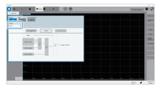
START<sup>™</sup> Starts recording when the instrument is triggered, and stops the recording after the instrument has acquired the recording-length waveforms.
