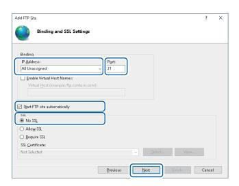
9 Configure the [Binding] and [SSL] settings as follows:
