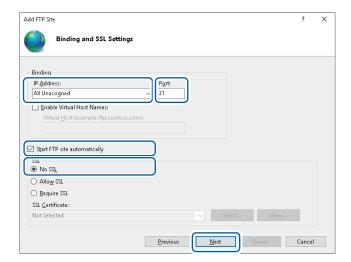
9 Configure the [Binding] and [SSL] settings as follows:
