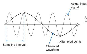
A sampling interval longer than the cycle of the input signal causes aliasing.
