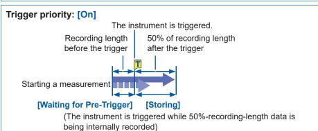
When the instrument is triggered while it is filling the pre-trigger memory, the length of the data actually recorded may be shorter than the specified recording length. (In this case, the pre-trigger recording length is shortened. The recording length after a trigger is calculated by subtracting the specified pre-trigger length from the specified recording length.)
