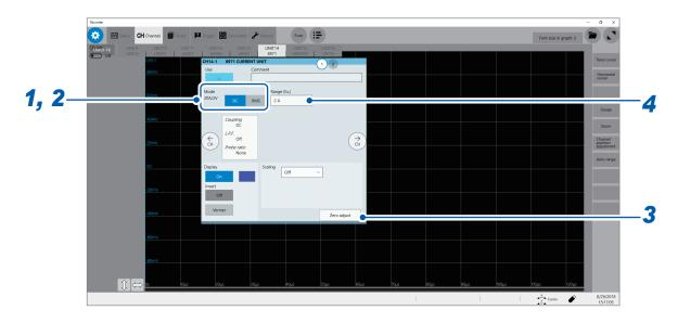
1 Confirm the output rate displayed in the [Mode] area.
