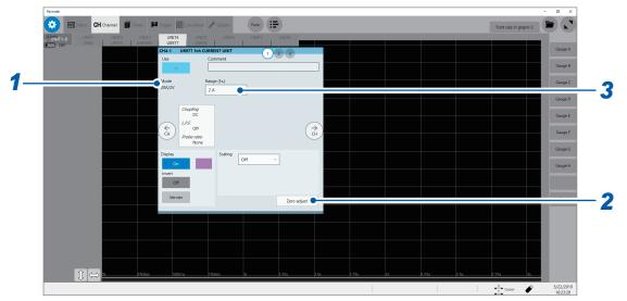
Current sensors to be connected determine whether the instrument automatically recognizes mode or whether you have to choose a current sensor setting.
