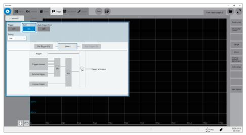
Setting [Alert] to [On] limits the sampling rate to 100 kS/s or lower. The event count of the trigger setting is fixed at 1.
