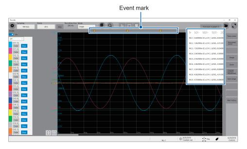
The instrument puts event marks () at the positions when the specified trigger condition is satisfied (alert issued) and when the condition fails to be satisfied (alert terminated). At the upper right of the screen, the instrument displays the time when the condition is satisfied, channel number, trigger type, measured value and a character string [Out] or [In].
