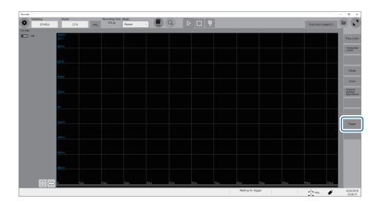
Clicking **[Trigger]** on the right side of the waveform screen allows you to manually trigger the instrument while the instrument is waiting time for a trigger.
