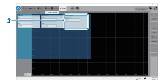
In the [External trigger] area, click the [Trigger out] box, and then from the list, choose a signal output method.
