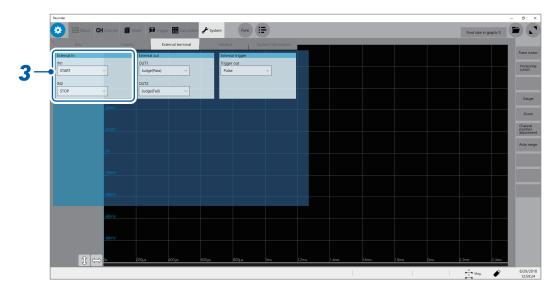
3 Click the [IN1] and [IN2] boxes in the [External In] area in turn, and then from the list, choose an action performed when an input signal is inputted.
