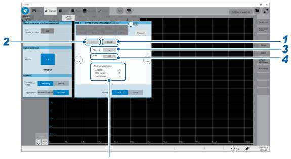
Displays the looping count, step number, and sweeping count of the still-in-progress process.
