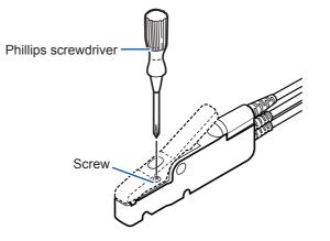
2 Adjust the stopper position by moving the stopper back and forth and tighten the screw.
