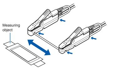
If the measurement is difficult, fixing can be done at the center. However, effectiveness of noise cancellation will reduce. (The return cable is indicated black in the illustration.)
