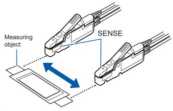
3 Adjust the position of the probes such that the return cable between the probes does not sag, and fix by pushing the return cable into the grooves of the probes.
