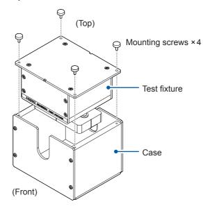
Remove the mounting screw found at each of the four corners on top of the fixture and remove the test fixture from its case.
