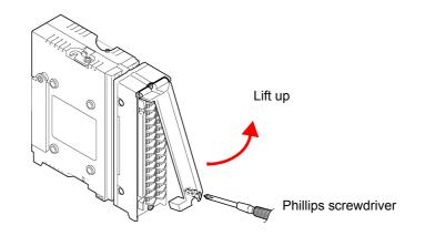
7. Loosen the screws of the terminal block, connect the input cable, and then tighten the screws.
