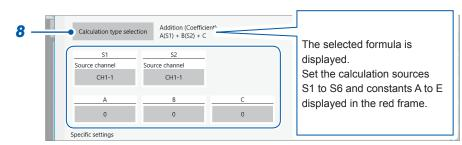
**3** Tap [Calculation type selection], and then choose a calculation type, calculation target channels, and calculation conditions.
