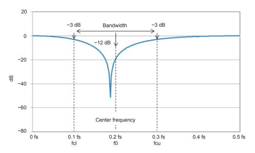
The bandwidth that can be set for the IIR band-stop filter varies depending on the center frequency.
