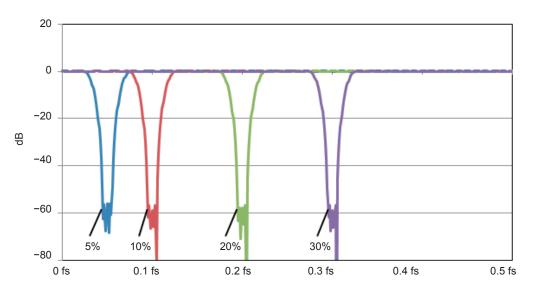
Example of FIR-BSF frequency characteristics (bandwidth: 5%)
