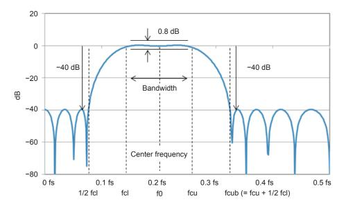
Where the center frequency of the band-pass filter is f0 and the bandwidth is fw, the lower passband edge (fcl) and the upper pass-band edge (fcu) are calculated by the following expressions: fcl = f0 - fw/2fcu = f0 + fw/2 The bandwidth that can be set for the FIR band-pass filter varies depending on the center frequency.
