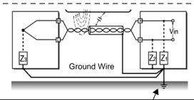
If the signal side is not grounded or if it is grounded inadequately, connect the HiLogger to ground. Also ground the shielding for the signal wires on the HiLogger side securely. Appendix
