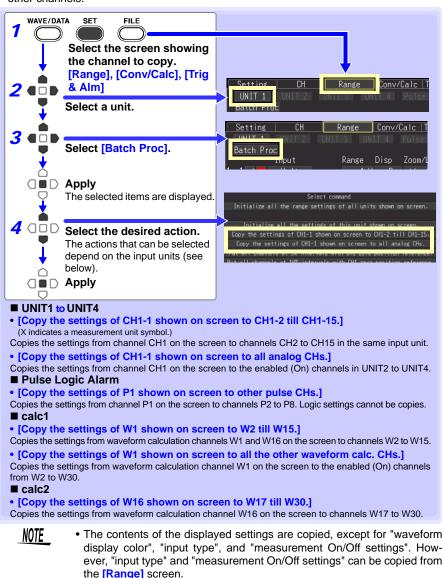
RTD (Resistance Temperature Detector) and resistance settings (specific to a Universal Unit) cannot be copied to a Voltage/Temperature Unit.
