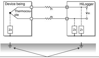
When using a thermocouple to measure temperature, noise can affect measurements unless both the device being tested and the HiLogger are grounded. Although there is no problem if the HiLogger is running on battery power, the HiLogger must be connected to ground if an AC adapter is being used.
