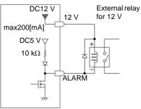
Example of an alarm output connection
