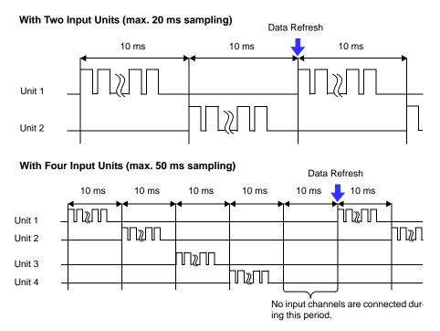
When the digital filter is off, the scan widths and dead times between channels are fixed to the values shown in the figure above regardless of the recording intervals. When the digital filter is on, the scan widths and dead times between channels vary in accordance with the recording intervals.
