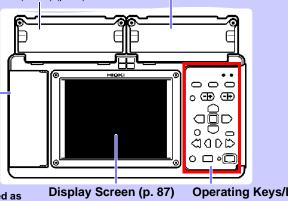
5.7-inch TFT color LCD Screen Configurations (p. 21) **Operating Keys/LED** (p. 19)
