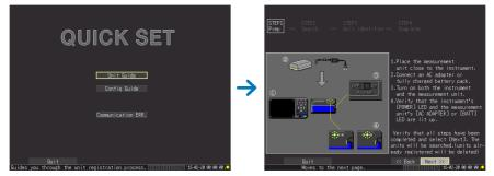
**3** Set the measurement conditions using the Quick Set function (Config Guide) and send the conditions to the instrument.
