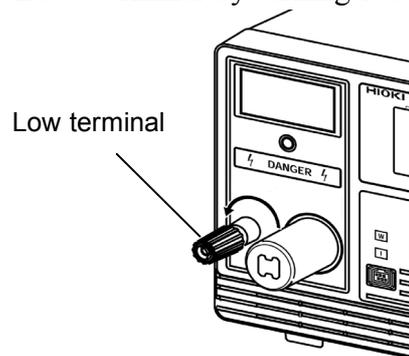
2. As shown in the figure, insert the plug on the H.V. TEST LEAD (low voltage side).
