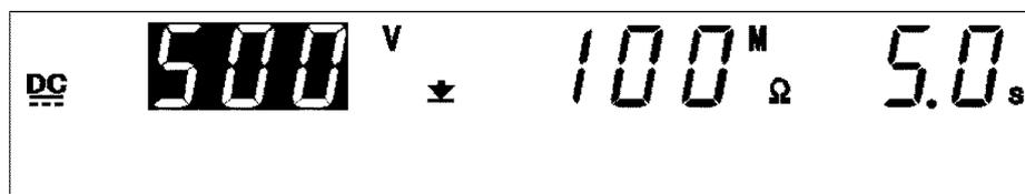
When the test conditions have been set, press the **ENTER** key. Pressing the **ENTER** key at this point finalizes settings (3) to (6). When the settings have been finalized, the step number selected in (3) is fixed as that for the settings.
