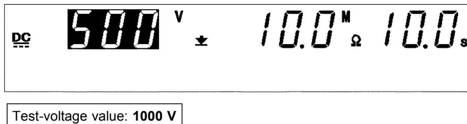
1. If no flashing cursor is displayed in the insulation-resistance mode READY state, press either the ◀/▶ key to display the cursor in the test-voltage value position.
