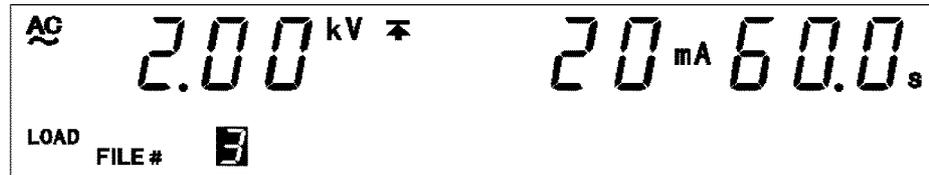
3. The "test voltage" and "test frequency" (in the case of AC-withstand-voltage) can be confirmed using the  $\blacktriangleleft$  key, the "upper-limit value" and "lower-limit value" can be confirmed using the  $\blacktriangleright$  key, and the "test time" and "ramp-up/down time" can be confirmed using the ON/OFF key.
