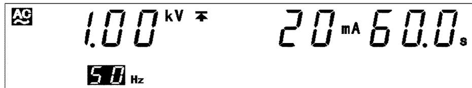
Test-voltage type: **AC 50 Hz**
