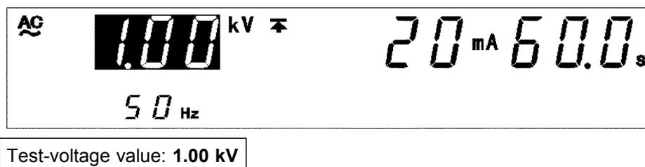
1. If no flashing cursor is displayed in the withstand-voltage mode READY state, press either the ◀/▶ key to display the cursor in the test-voltage value position.
