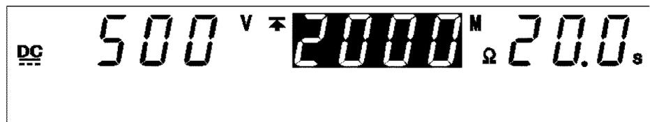
The upper-limit value is set at 2000 M $\Omega$ . Turn it **OFF**, as it is not needed. To change to **OFF**, press the **ON/OFF** key.
