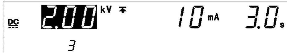
When the test conditions have been set, press the **ENTER** key to finalize the settings. Press the **STOP** key to exit the program setting state. The unit will change to the program mode and enter the READY state. File 2 is set as follows:
