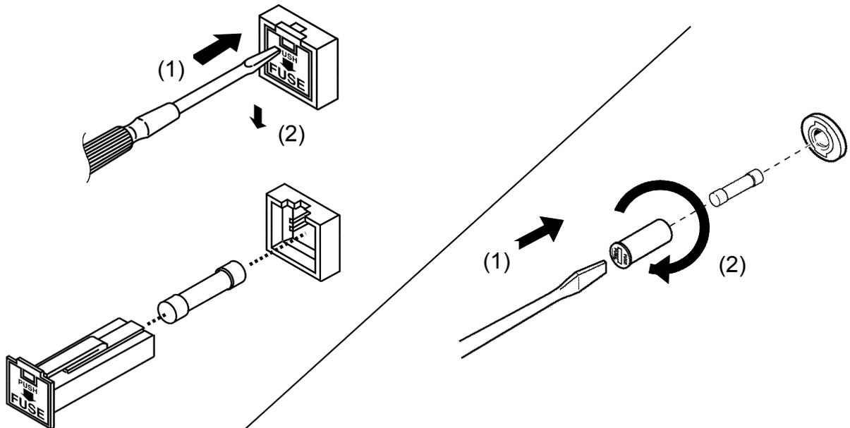
3. Replace the power fuse with a rated fuse. (The replacement method may differ depending on the shape of the fuse holder.)
