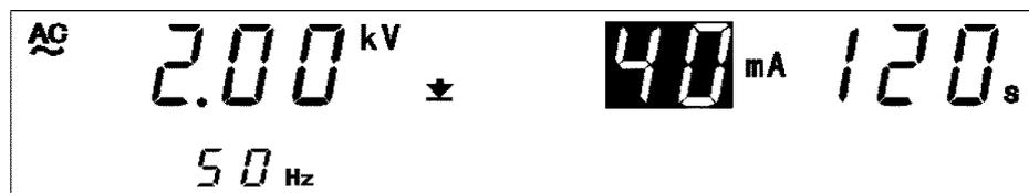
The lower-limit value is set at **40 mA**. Turn it OFF, as it is not needed. To change to OFF, press the **ON/OFF** key.
