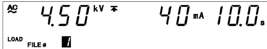
At this time, the "test frequency" (in the case of AC-withstand-voltage) can be confirmed using the **◀** key, the "lower-limit value" can be confirmed using the **▶** key, and the "ramp-up/down time" can be confirmed using the **ON/OFF** key.
