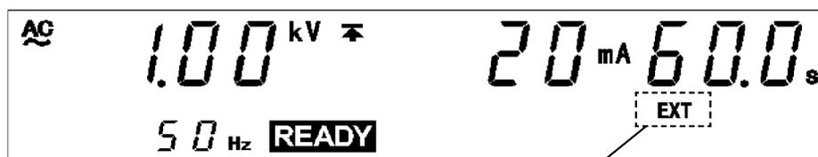
When EXT-E of the external I/O terminal is at LOW level, EXT lights up when the REMOTE CONTROL BOX is active.
