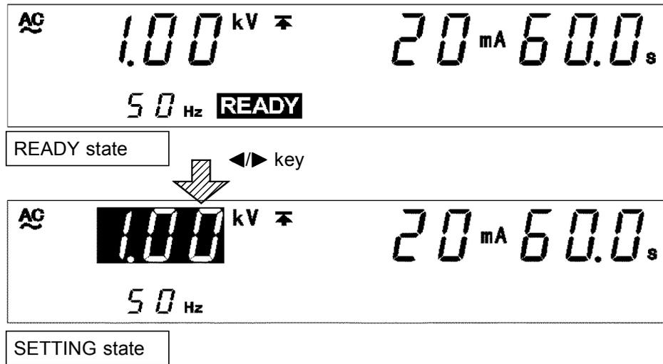
1. In the withstand-voltage mode READY state, when you press the  $\leftarrow/\rightarrow$  keys, the flashing cursor appears where the test voltage is indicated to show that the unit is in the SETTING state. (The **READY** light goes out and tests cannot start even if the **START** key is pressed.)
