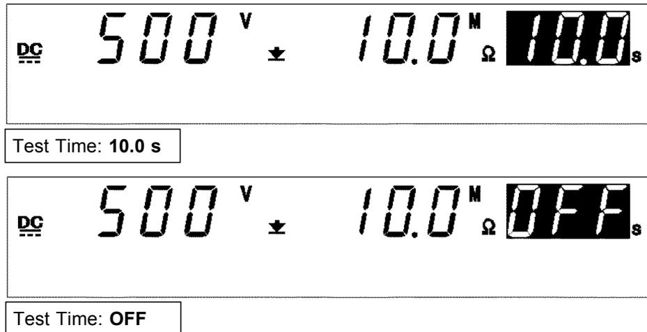
1. If no flashing cursor is displayed in the insulation-resistance mode READY state, press either the ◀/▶ key to display the cursor in the test time position.
