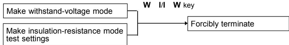
If you try to start a test in the Auto test mode, the test mode when the test time is switched **OFF** is displayed (**OFF** flashes), and the test cannot be started.
