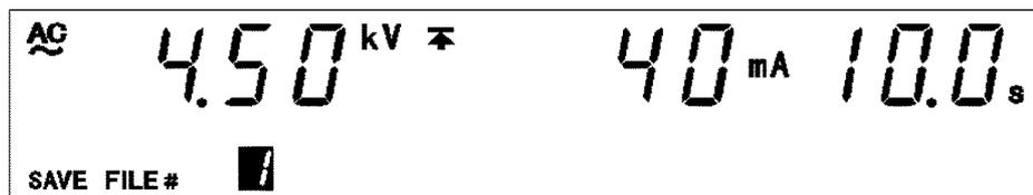
At this time, the "test frequency" can be confirmed using the **◀** key, the "lower-limit value" can be confirmed using the **▶** key, and the "ramp-up/down time" can be confirmed using the **ON/OFF** key.
