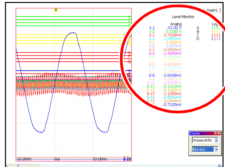
[Monitor] The Level Monitor value of each waveform is displayed. Levels can be displayed.(p. 199)
