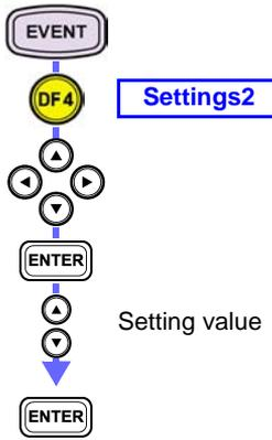
The diagram shows a vertical sequence of controls: an 'EVENT' button, a yellow 'DF4' button, a 'Settings2' label in a blue box, a set of four directional arrow buttons (left, up, down, right), an 'ENTER' button, another set of four directional arrow buttons, and a final 'ENTER' button. A blue arrow labeled 'Setting value' points from the second set of arrow buttons to the 'ENTER' button below it.
