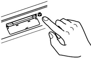
Press the Eject button and pull the PC Card out.
