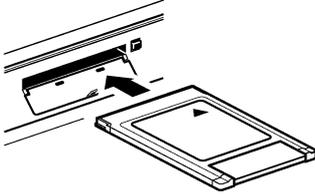
Open the cover and insert the PC Card with the arrow facing up and in the direction of the PC card slot, as far as it will go.
