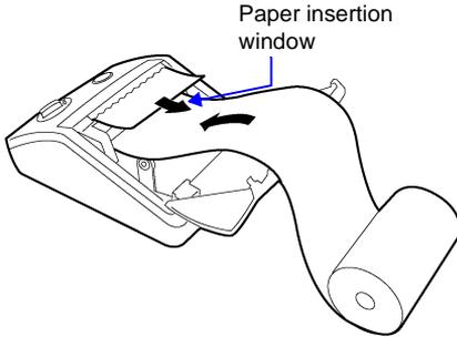
Load the recording paper into the 9670 PRINTER.
