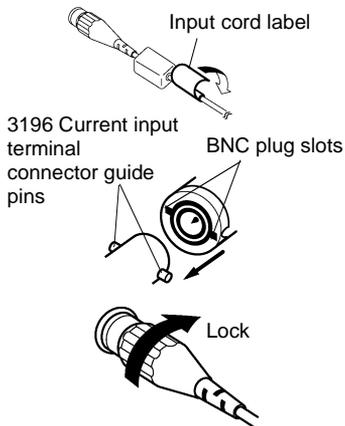
1. At each end of the cable, apply the labels having the same color as the current input terminal to which it is to be connected.
