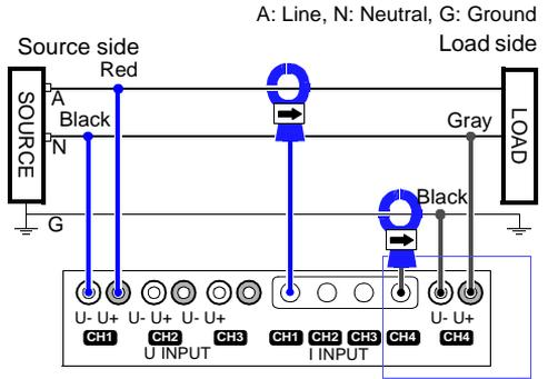
⇒ Face the arrow toward the Load Ground line measurement, etc.
