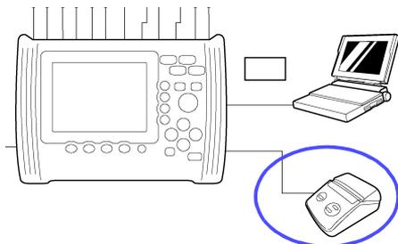
The instrument can produce hard copies of the screen on the Model 9670 PRINTER connected to the RS-232C interface.
