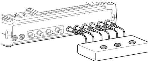
Connect all six output leads from the Wiring Adapter to the voltage input terminals with the corresponding colors on the instrument.
