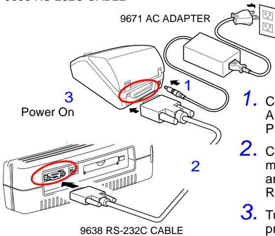
1. Connect the 9671 AC ADAPTER to the 9670 PRINTER.
