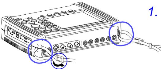
1. Insert each end of the Strap through an installation slot on the instrument.
