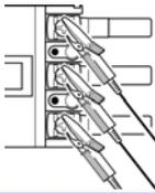
Clip securely to metal parts such as connection screws or bus bars at the power side.
