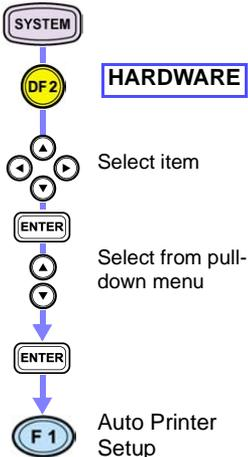
The 9670 PRINTER is automatically set up for use by the instrument.
