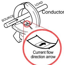
The arrows on the clamp indicating the direction of current flow should point toward the load side.
