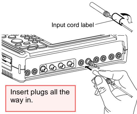
1. At each end of each cord, apply the labels that correspond to the (same-color) input terminal to which it is to be connected.
