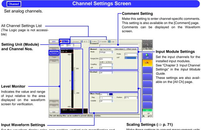
Set the waveform display color, zero position, vertical axis magnification and display area. These settings are also available on the [All Ch] page.
