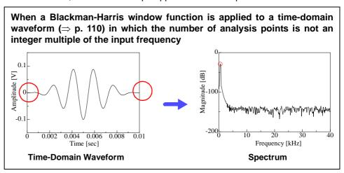
The following figure shows the time-domain waveform of the window function and its spectrum.
