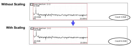
Setting example: To display measurement data on this instrument so that it corresponds to that on a sound level meter.
