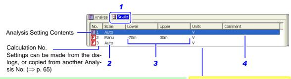
2 Select automatic or manual scaling of the y-axis display.
