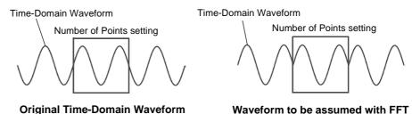
When the number of points for FFT analysis is an integer multiple of the input signal frequency, a single-line spectrum is obtained. However, if it is not an integer multiple of the frequency (when the waveform assumed with FFT includes discontinuous points), the spectrum is scattered, and a line spectrum cannot be obtained. This phenomena is called leakage error (as shown below).
