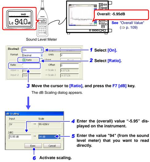
Scaling is performed automatically, and the corresponding values appear in the conversion ratio fields.
