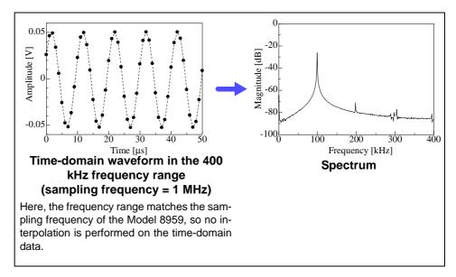
To avoid imaging phenomena when analyzing waveforms with the FFT function, verify the maximum sampling frequency of the input module before measuring.
