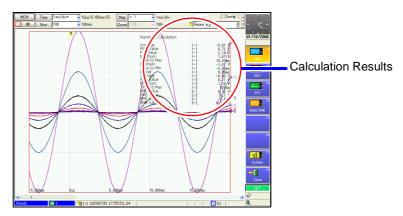
If the display is hard to view because of overlapping numerical values and waveforms Press the **DISP** key. Numerical values and waveforms are displayed separately.
