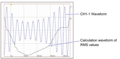
To view the waveform calculated from the acquired data, press the [Execute] button on the Waveform Calculation Settings screen.
