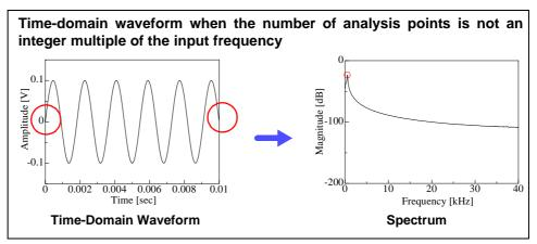
The window function was created to suppress such leakage errors. The window function smoothly connects each end of the time-domain waveform where it is cut off.
