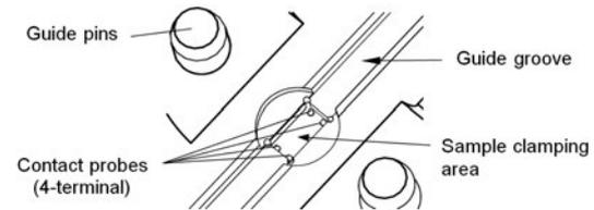
Fig. 2. Sample Clamping Sub-unit
