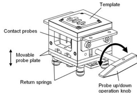
Fig. 3. Test Head Unit
