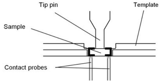
Fig. 1. Sample Electrode and Probes
