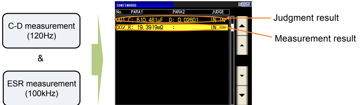
Measurement and Judgment example of continuous measurement function.
