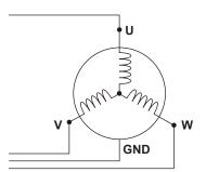
Object under measurement is a neutral pointconnected three-phase stator
