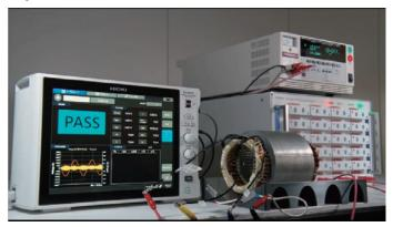
**2** Connect the cables of the calibration pulse generator to U and V on the object under measurement.
