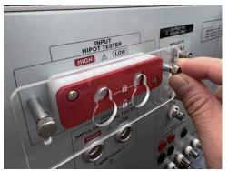
**4** Slide up the cable dropout prevention plate.
