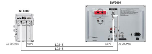
**3** Connect the SW2001 and the withstand voltage tester.
