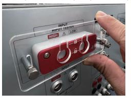
**5** Align the connection cable connectors with the terminal holes and insert them all the way inside.
