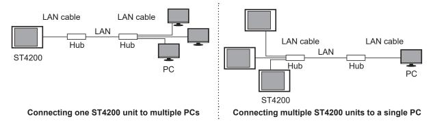
Use either a commercially available 100BASE-TX or 10BASE-T LAN cable. Either a straight-through cable or crossover cable can be used.
