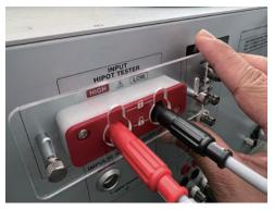
**6** Slide down the cable dropout prevention plate until it comes in contact with the screws and locks the connectors in place.
