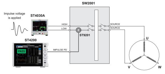
When the object under measurement is a neutral point-connected three-phase stator
