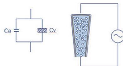
Fig. 11. Model diagram and equivalent circuit: with varnish
