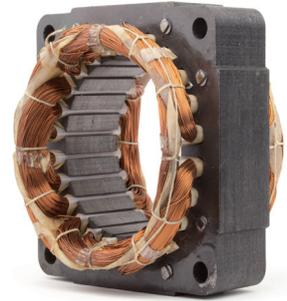
There are two types of varnish impregnation treatments: trickle impregnation, in which the coil is immersed in a tank of varnish (which serves as an insulating material), and vacuum impregnation, in which varnish is injected after the coil is subjected to a vacuum.
