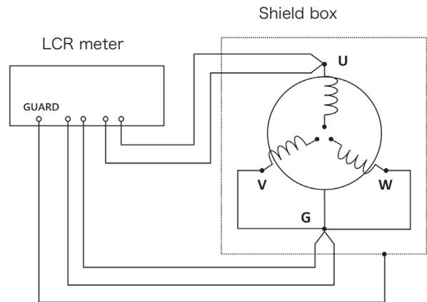
Fig. 5. Example test circuit (U-VWG)
