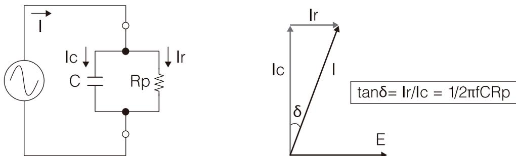
Fig. 1. Electrical equivalent circuit of an insulator and vectors when an AC voltage is applied
