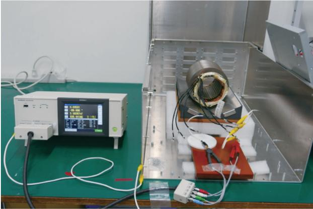
Fig. 2. LCR meter and measurement setup
