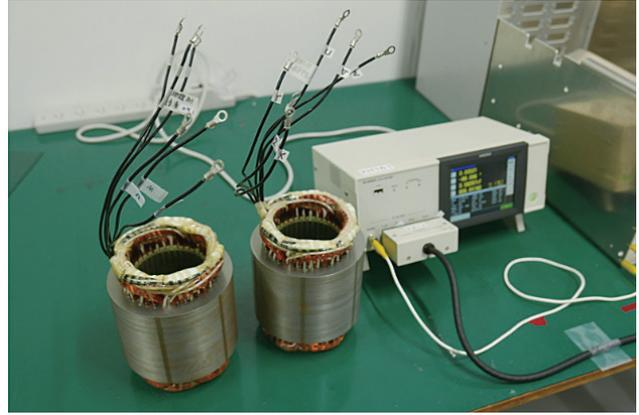
Fig. 3. Samples with different amounts of impregnation
