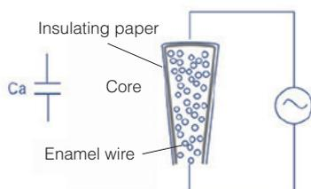
Fig. 10. Model diagram and equivalent circuit: without varnish
