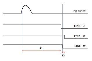
Illustration of circuit breaker operation measurement results
