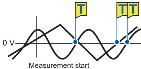
The trigger is activated when one crosses 0 V from below to above.
