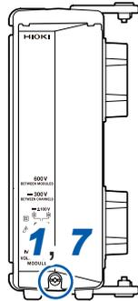
**1** Remove the screw for the terminal block cover.
