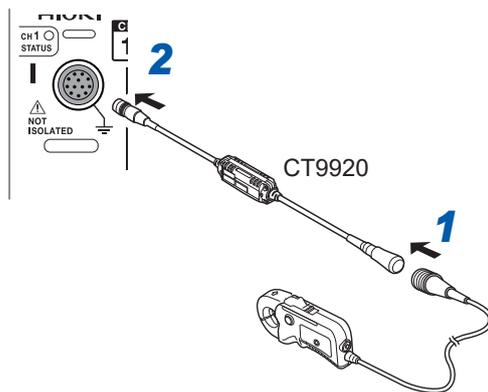
**1** After turning OFF the instrument, connect the CT9920 conversion cable by aligning it with the connector guide of the current sensor.
