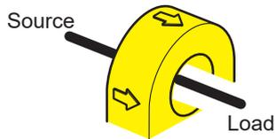
Clamp the current sensor onto the wire with the current direction arrow pointing towards the load side.
