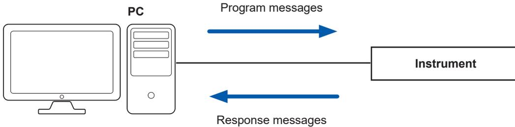
The data sent and received between communication devices is referred to as a message. The messages are categorized as shown in the figure below.
