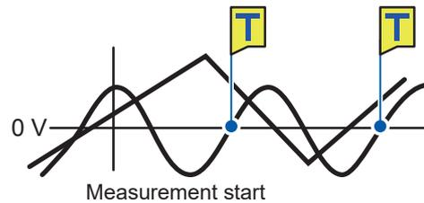
The trigger is activated when one is above 0 V and the other crosses 0 V from below to above.
