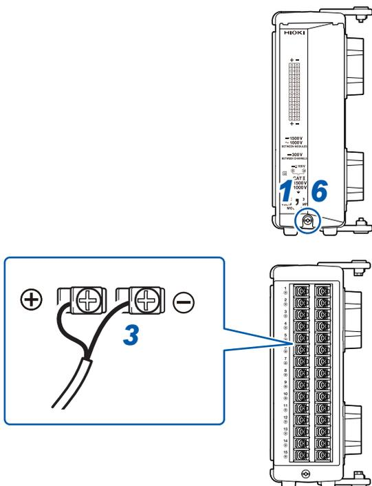
**1** Remove the screw for the terminal block cover.
