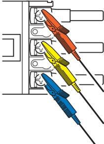
Securely clip the voltage cords to the relevant metal part, such as the screw and wiring bar on the power supply side.
