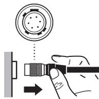
**1** While holding the metal part of the connector, release the lock by sliding it to the cable side.
