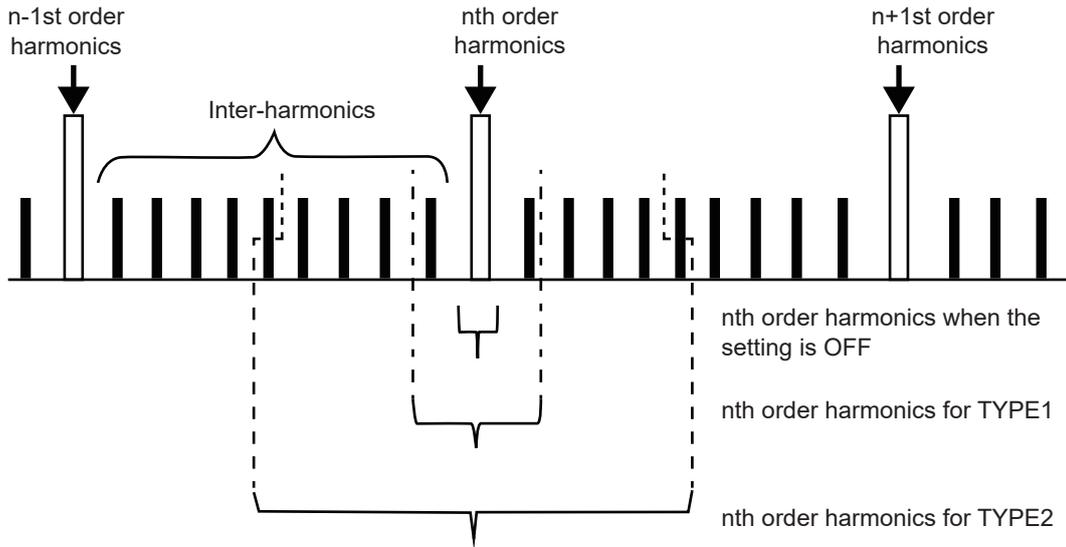
Usually, TYPE1 range is called “harmonic sub-group”, and TYPE2 range is called “harmonic group”. Each range can be calculated by square-root of sum of squares of the output bins within the range. If there are no inter-harmonics or the window wavenumber is 1 in a wide area mode, the measurement values will be consistent regardless of which grouping method is selected. If inter-harmonics are present, the relationship of the harmonic measurement values will usually be “OFF < TYPE1 < TYPE2”.
