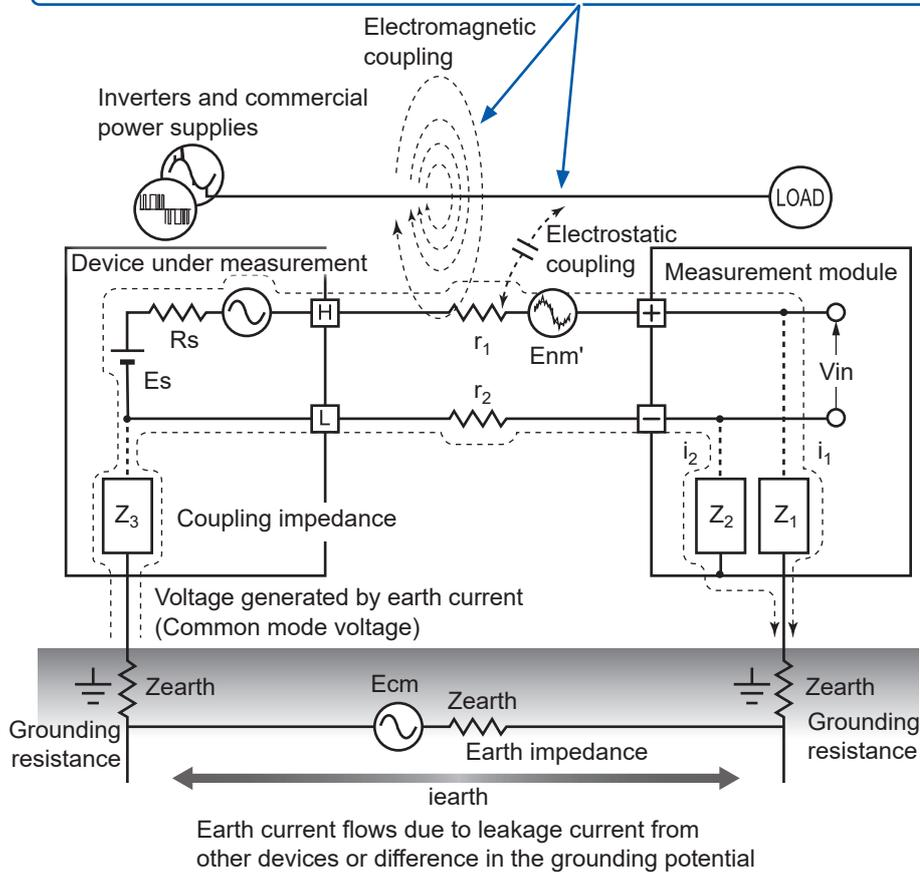
Common mode noise occurs when the earth impedance intervenes between the grounding point of the device under measurement and the grounding point of the measurement module, or if the earth line is coupled capacitively with a noise source.
