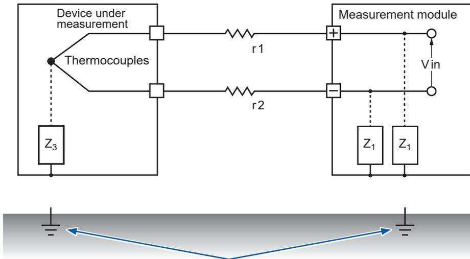
Temperature measurement using a thermocouple is affected by noise unless both the instrument to be measured and the measurement module are connected to the ground. Be sure to ground the AC adapter when using it.
