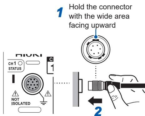
**1** After turning OFF the instrument, align it with the connector guide of the current sensor.
