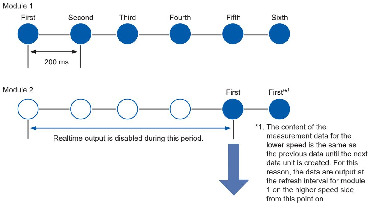
The measurement data do not progress until the lower speed data become ready. Once the lower speed data become ready, the data for both the higher speed and lower speed will progress. At this point, the initial data of the summarized data is output. (The first to fifth data units of module 1 and the first data unit of module 2 in the above drawing)
