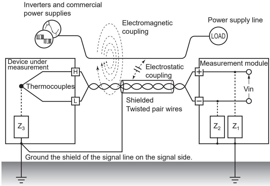
Keep away and separate the signal lines (thermocouples) from the wiring that can be noise sources (power lines, etc.). Furthermore, electrostatic coupling can be blocked by shielding and grounding the signal lines.
