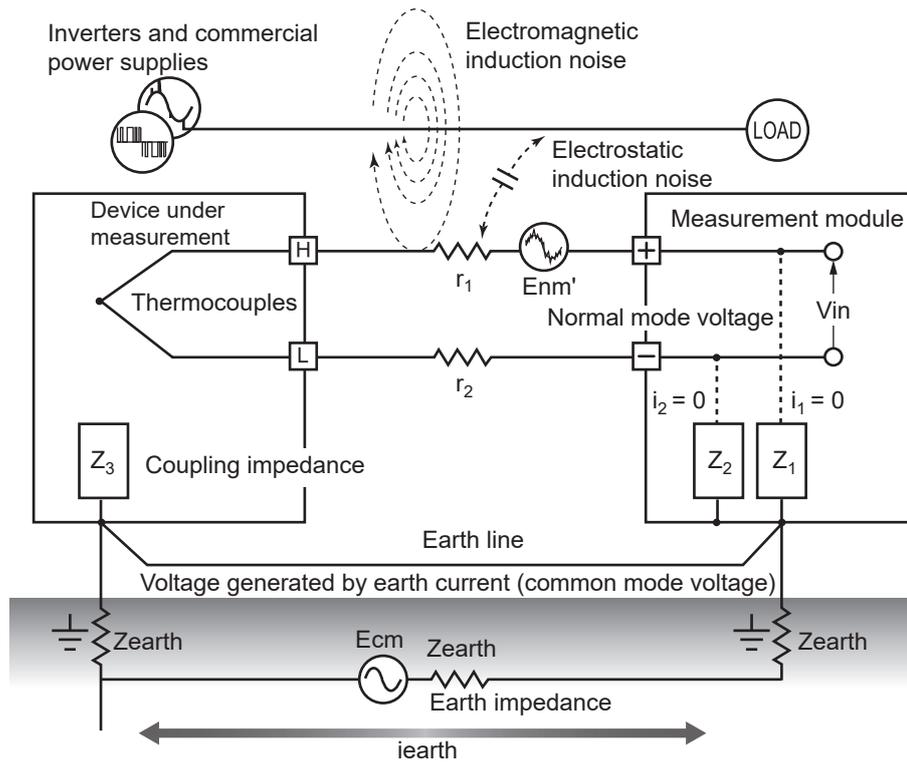
Ground the chassis GND on the signal side to a good earth with a sufficiently low grounding resistance.
