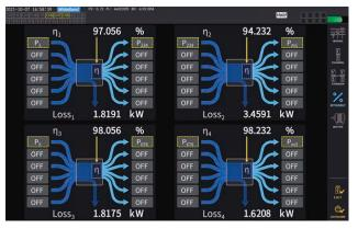
The results indicate that the front motor (Pm1) has a somewhat low efficiency of 94.2% and that 3.4 kW of loss is occurring.
