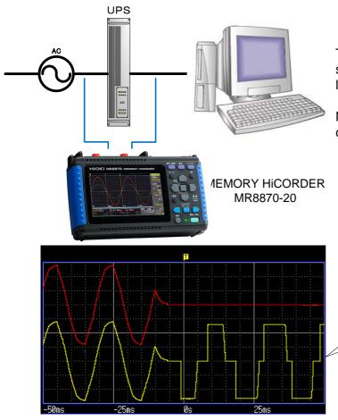
CH1 (red) shows the primary utility power supply voltage waveforms and CH2 (yellow) shows the secondary voltage waveforms of the UPS system.
