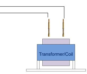
Coils and transformers, which must deliver a high level of reliability, are subject to insulation resistance measurement, dielectric withstand testing, resistance measurement, and impulse testing.
