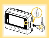
Align the triangle on the plug with the one in front of the sensor jacks, and insert the plug securely.
