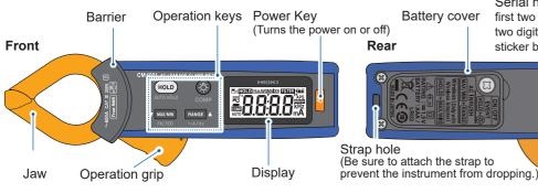
Serial number (The serial number consists of nine digits. The first two digits indicate the year of manufacture, while the second two digits indicate the month of manufacture. Do not remove this sticker because the number is important.)
