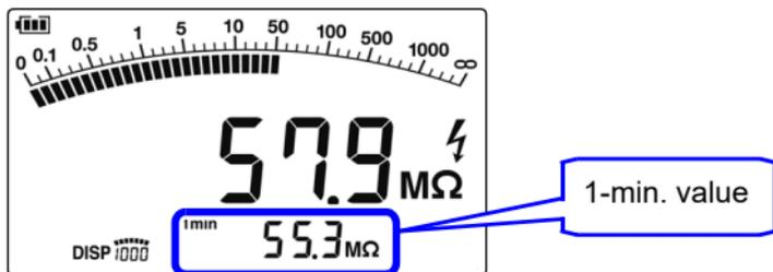
Use this function when measuring targets that include a capacitance component.
