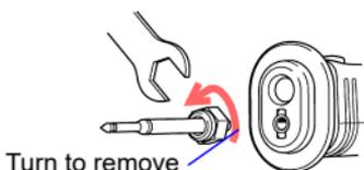
3. Turn the new tip pin with a spanner and attach it to the L9788-10. (tightening torque:  $0.3\text{N}\cdot\text{m}$ )
