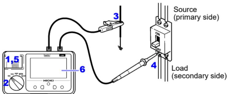
Ex. When measuring the insulation resistance between circuit and ground
