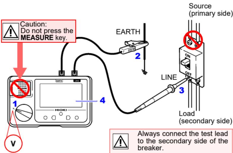
Ex. When measuring the voltage between circuit and ground
