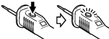
6. Press LIGHT of the instrument to confirm that the light at the tip of the L9788-10 comes on.
