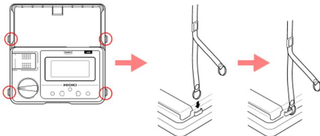
Pass the ring on both ends of the supplied strap through each of the four holes in the instrument.
