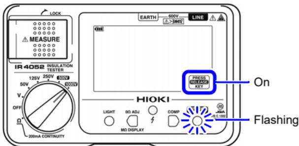
2. Press  to turn off  or  as well as  , disabling the lock. The display will also change as  , to the measurement screen.
