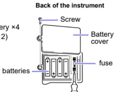
1. Turn the rotary selector to OFF and remove the test lead from the instrument as a precaution.
