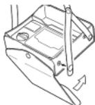
Undo the snap fastener on OPEN mark side. Lift the cover and pivot it to the side and under the case itself and redo the snap fastener on the side of the cover.
