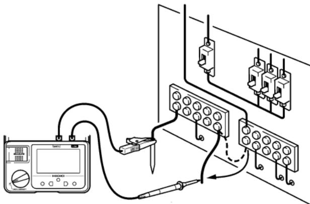
Ex. Checking the continuity of ground wiring
