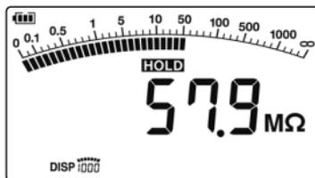
**NOTE** Measurement of a solar panel may fail to turn off ⚡ because the voltage generated by the solar panel is detected after completely discharged.
