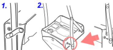
1. Undo the snap fastener for the strap on the left side of the case.
