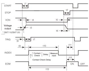
t0: 0.1 ms or greater, t1: 0.1 ms or greater, t3(t6): delay, t7: 0.1 ms or greater t4 (t5): Voltage output (stop) time: Less than 0.1 ms, t8: Trigger accepted: 0 s or greater t9: INDEX, EOM delay time, t10:INDEX time, t11: START setup time: 4 ms or greater t12: TRIG setup time: Display ON (40 ms or greater) Display OFF (1 ms or greater) t13: EOM time
