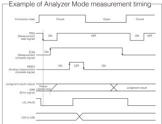
EOM: Off from trigger input to end of measurement processing INDEX: Off during probe chuck (probe cannot be removed from target)
