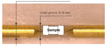
Shape of probe tip: 60° cone
