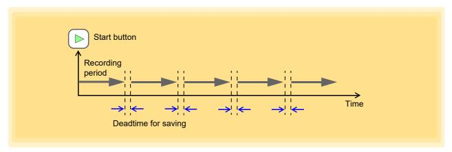
If you set a repeat measurement interval for timer measurement (p. 72), it is possible to repeat measurement while leaving a gap at a fixed interval as shown in the figure below.
