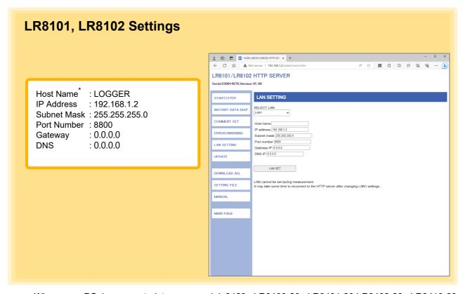
When one PC is connected to one model 8423, LR8400-20, LR8401-20,LR8402-20, LR8410-20, LR8450, LR8450-01, LR8101, or LR8102 using the crossover adapter supplied with the 9642 LAN Cable, any IP address can be specified. However, we recommend using private IP addresses. Enter a host name and IP address on the Logger that will not be duplicated on the PC.
