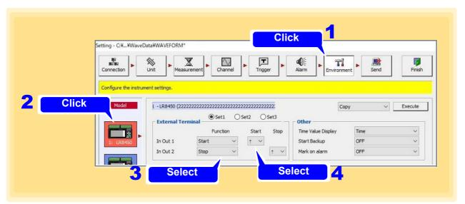
5. Select Set2, Set the InOut3 terminal function of the external control terminal.
