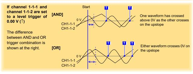
A trigger is not applied if the trigger criteria is already satisfied when measurement starts. If the criteria of one of the trigger sources is no longer satisfied and then the criteria is satisfied again, a trigger is applied.
