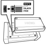
6 With the battery case facing down, fit it into the recessed area on the instrument.
