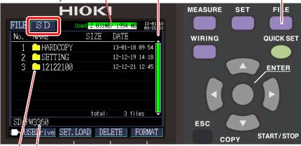
Displays the current display location. In this case, the screen is displaying the PW3360 folder on the SD memory card.
