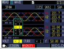
3 Select the desired zoom factor with the cursor's ( keys and press the (ENTER) key.
