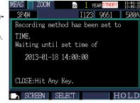
When the set start time is reached, recording will start (and the 3 RECORDING LED will light up).
