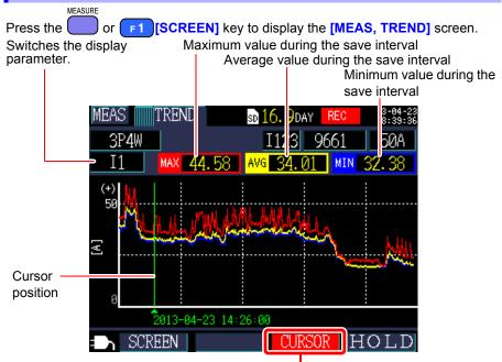
The cursor keys can be used to move the cursor. When the cursor is selected, time-series display updates stop.
