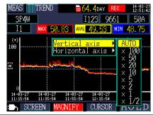
3 Select the desired zoom factor with the cursor keys and press the [ENTER] key.
