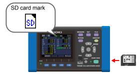
2 Display the screen you wish to save and press the You can save a hold screen by pressing the F4 [HOLD] key.
