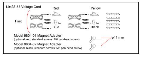
Voltage cords used by wiring type
