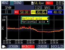
2 Select either [Vertical axis] or [Horizontal axis] with the cursor and press the ()[ENTER] key.
