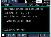
3 Recording will start automatically when a good time division is reached based on the save interval time.
