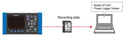
To access data, either load it from the SD memory card on which it was saved using a computer with an SD memory card reader, or use a USB cable to copy data from the SD memory card or internal memory to the computer.
