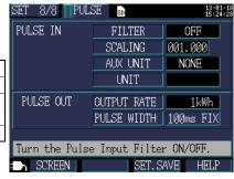
Filter ON (mechanical contact use):
