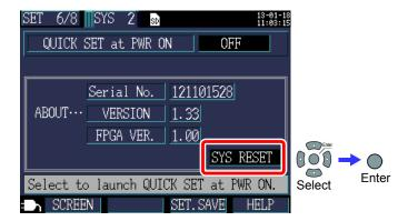
Performing a system reset causes all settings other than the frequency setting, clock, language setting, IP address, subnet mask, and default gateway to be initialized to their default values. The instrument's internal memory will not be erased.
