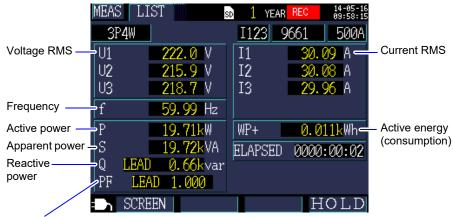
Selects between power factor PF (RMS calculation) and displacement power factor DPF (fundamental wave calculation) with settings.
