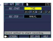
2 START/STOP Press the key on the Measurement screen.
