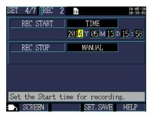
3 Change the setting with the \_\_\_\_/\_ cursor keys and then accept the new value with the \_\_\_ [ENTER] key.
