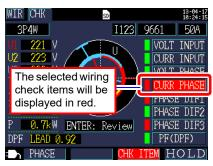
Move the cursor to the item that has been tagged as red (FAIL) or yellow (CHECK) and press the IENTER] key
