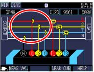
Connect the voltage sensor to the measurement target while checking the wiring target on the [WIR, DIAG] screen.
