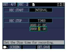
Change the setting with the cursor keys and then accept the new value with the [ENTER] key.
