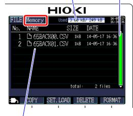
Displays the File screen and switches screens (SD memory card/internal memory).
