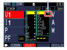
Select the desired parameter with the cursor keys and accept the new setting with the [ENTER] key.
