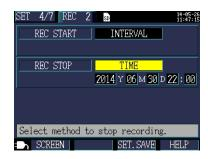
Once recording has been started and the set recording stop time is reached, recording will stop automatically. (and the recording LED On)
