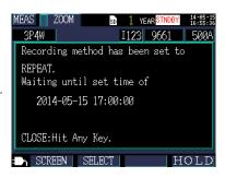
Recording will be started at the start time on the set start date. (The recording LED will light up.)
