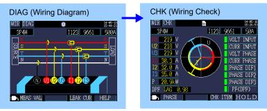
See: "Chapter 3 Connecting to Target to be Measured" (p.43)
