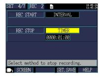
2 Once recording has been started and recording will stop automatically when the set timer time elapses. (and the recording LED On)
