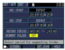
7 Select the folder creation timing with the cursor / keys and accept the setting with the [ENTER] key.
