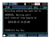
Recording will start automatically when a good time division is reached based on the save interval time. (and the recording LED will light up). Example
